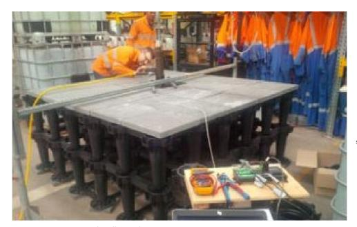
Figure 4.23 Strata vault cell sample
