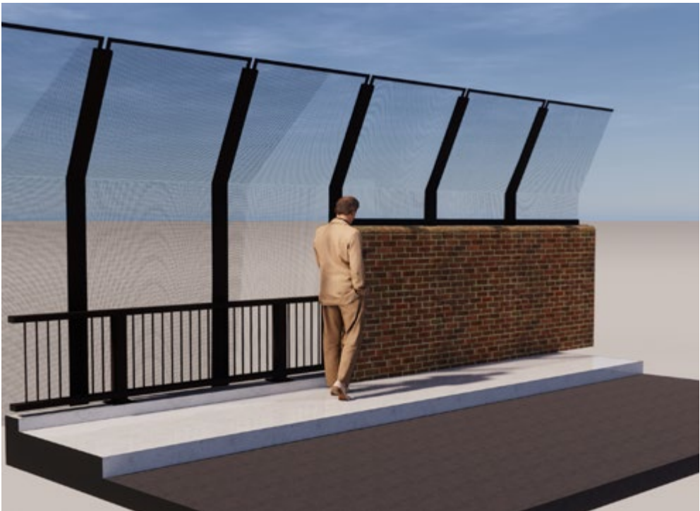
Figure 4.27 Typical vertical screen profile to Duntroon Street Bridge
