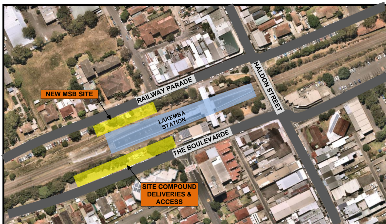
Figure 8 – Lakemba Station compound layout (Source: Near Map)
