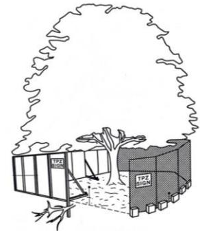
Where approved works are required within the TPZ, fencing may be setback to provide construction access. Trunk, branch, and ground protection shall be installed and must comply with Australian Standard, AS 4970-2009, Protection of Trees on Development Sites. Any additional construction activities within the TPZ of the subject trees must be assessed and approved by the project arborist.
