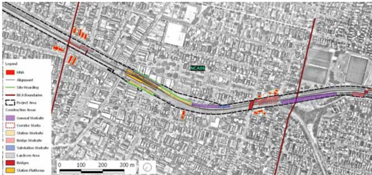
Figure 22 Highly Noise Affected Residential Receivers
