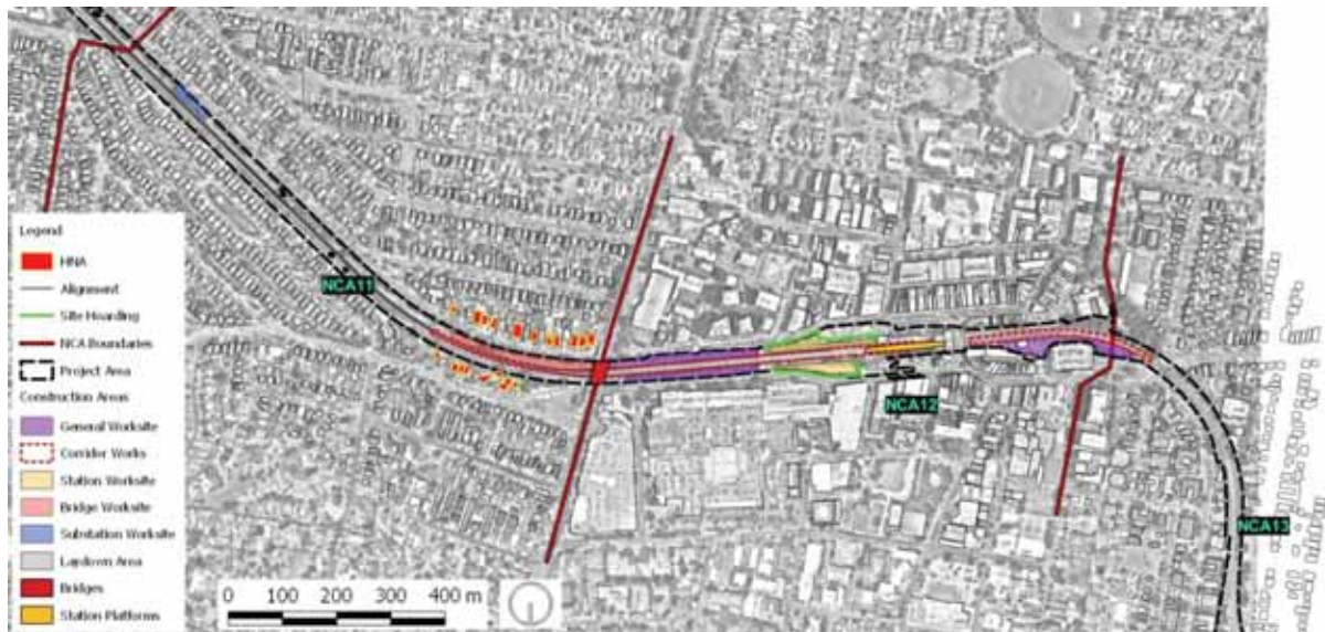
Figure 42 Highly Noise Affected Residential Receivers
