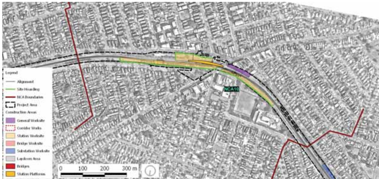
Figure 35 Punchbowl Precinct – Construction Areas
