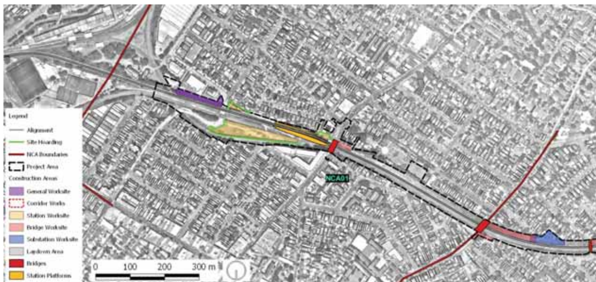
Figure 1 Marrickville Precinct - Construction Areas
