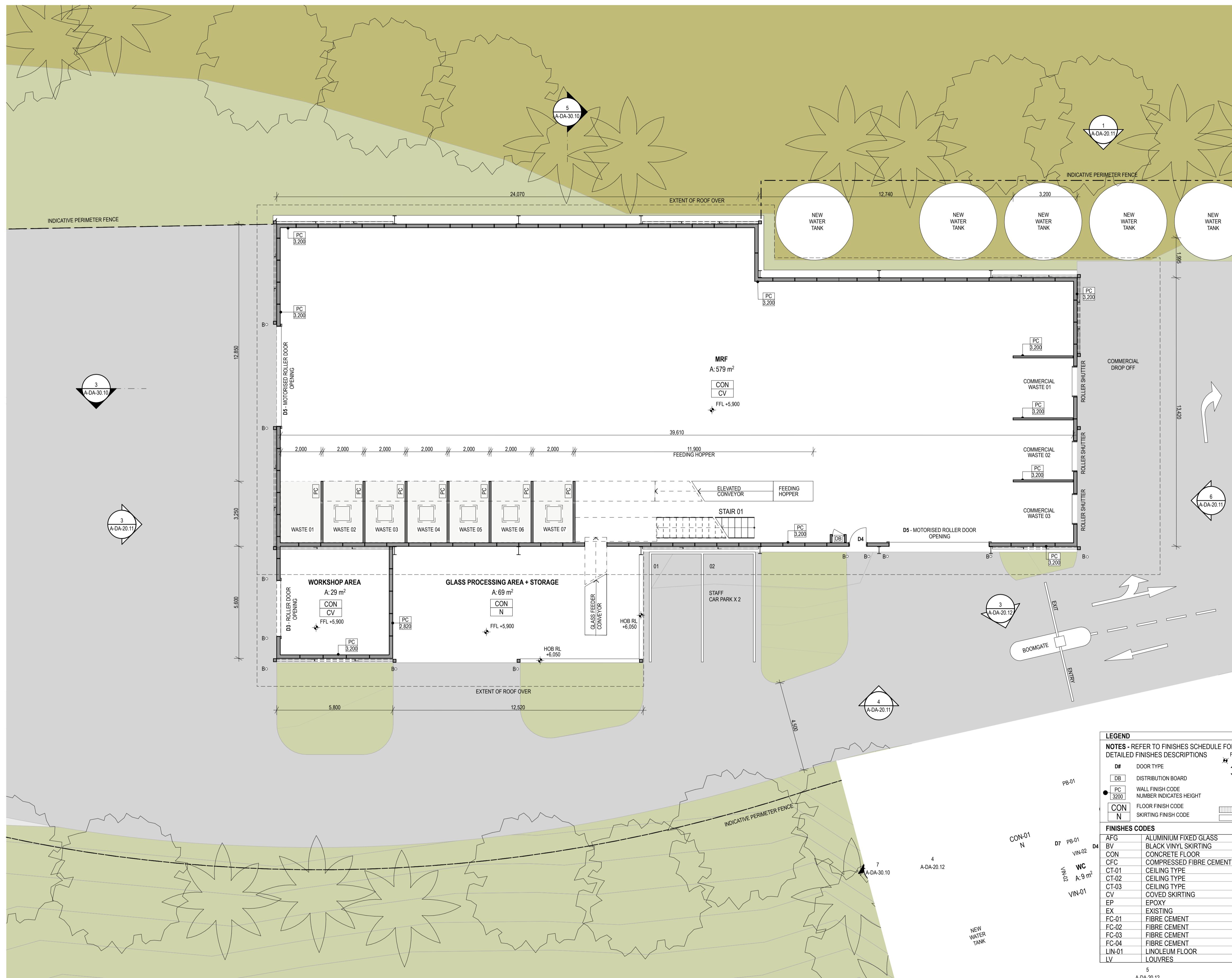
1 GROUND FLOOR PLAN - SOUTH ZONE (MRF + RECEPTION) 1:100
