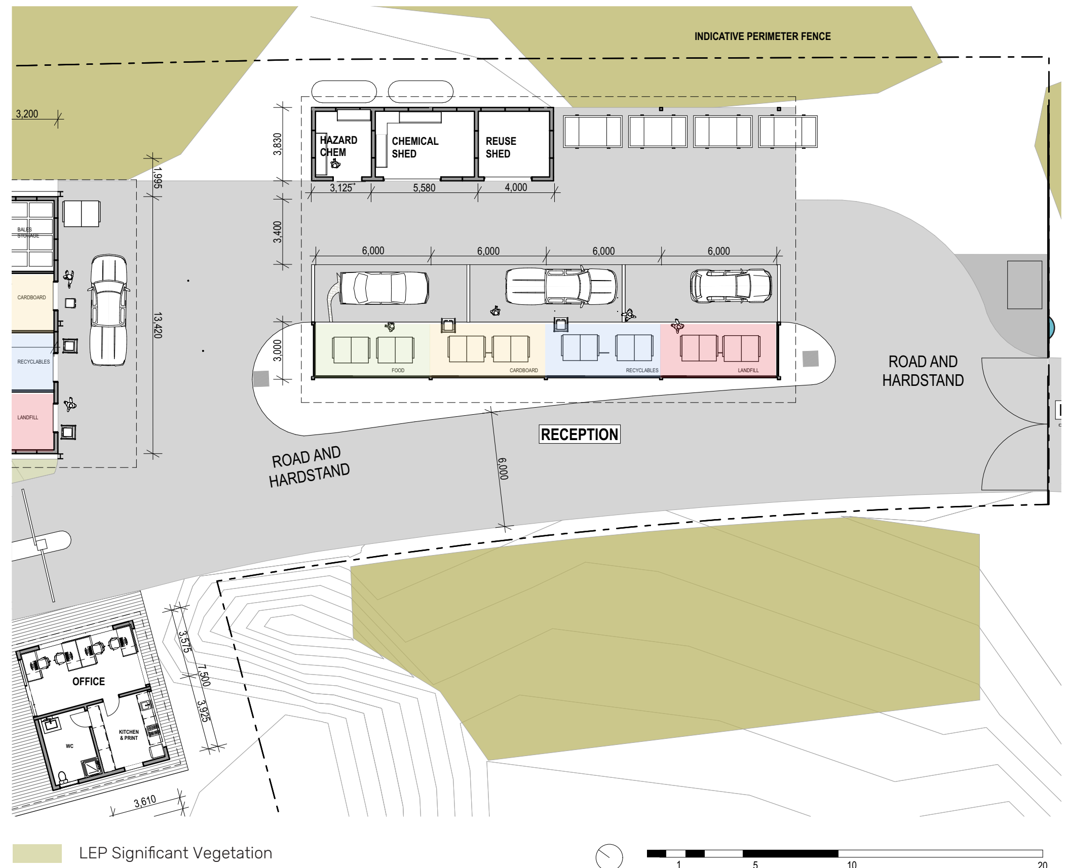
Figure 65: WMF Drop Off Area and Chemical Shed
