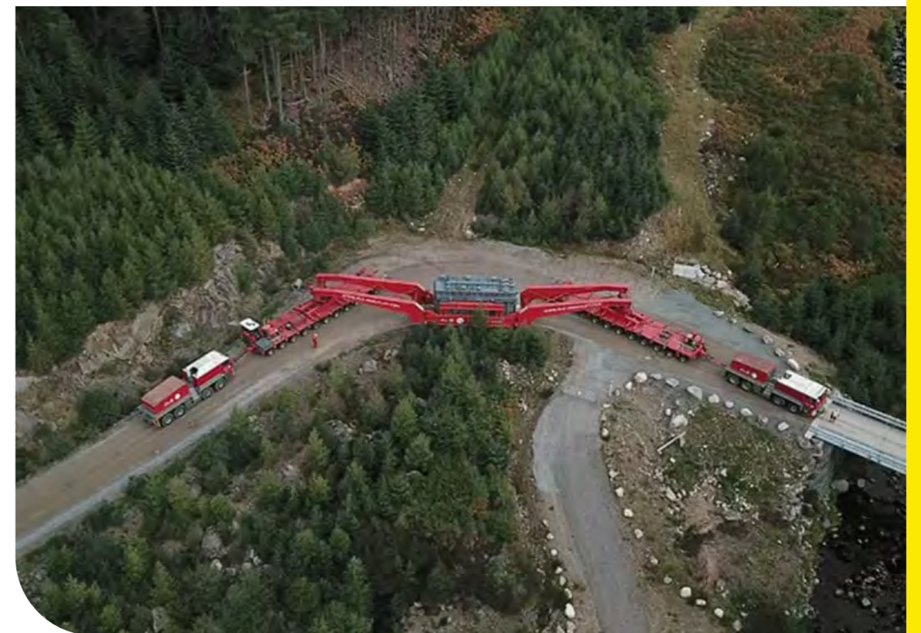
Above: Example of beam set used for large power transformer transport.
