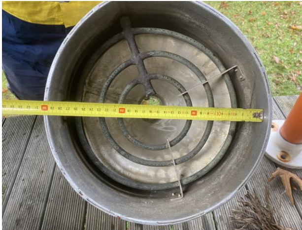
Figure 10: Airlift sampler used to sample macroinvertebrates (tape for scale)
