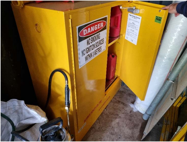
Image 5: Opal Blvd utility relocations (self-bunded chemical storage cabinet)
