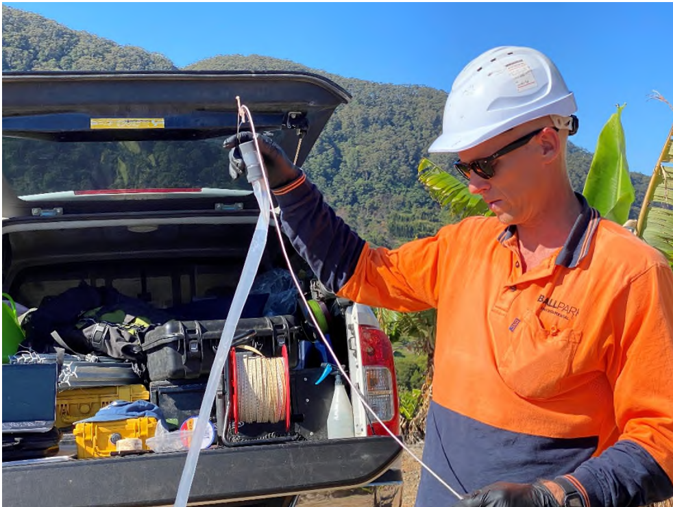
Photograph 4 , Hydrasleeves were installed in monitoring well locations at each of the tunnels to collect water samples for laboratory analyses.
