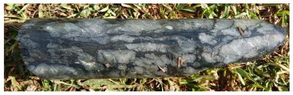
Photograph 8 Core from BHH127 showing ptygmatically folded quartz veins
