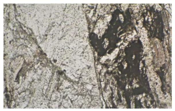
Photograph 3 Thin section cut from core from BHH132 27.46m-27.63m showing where three different textural and mineralogical 'types' are juxtaposed. Scale: side of photograph is 1.6mm
