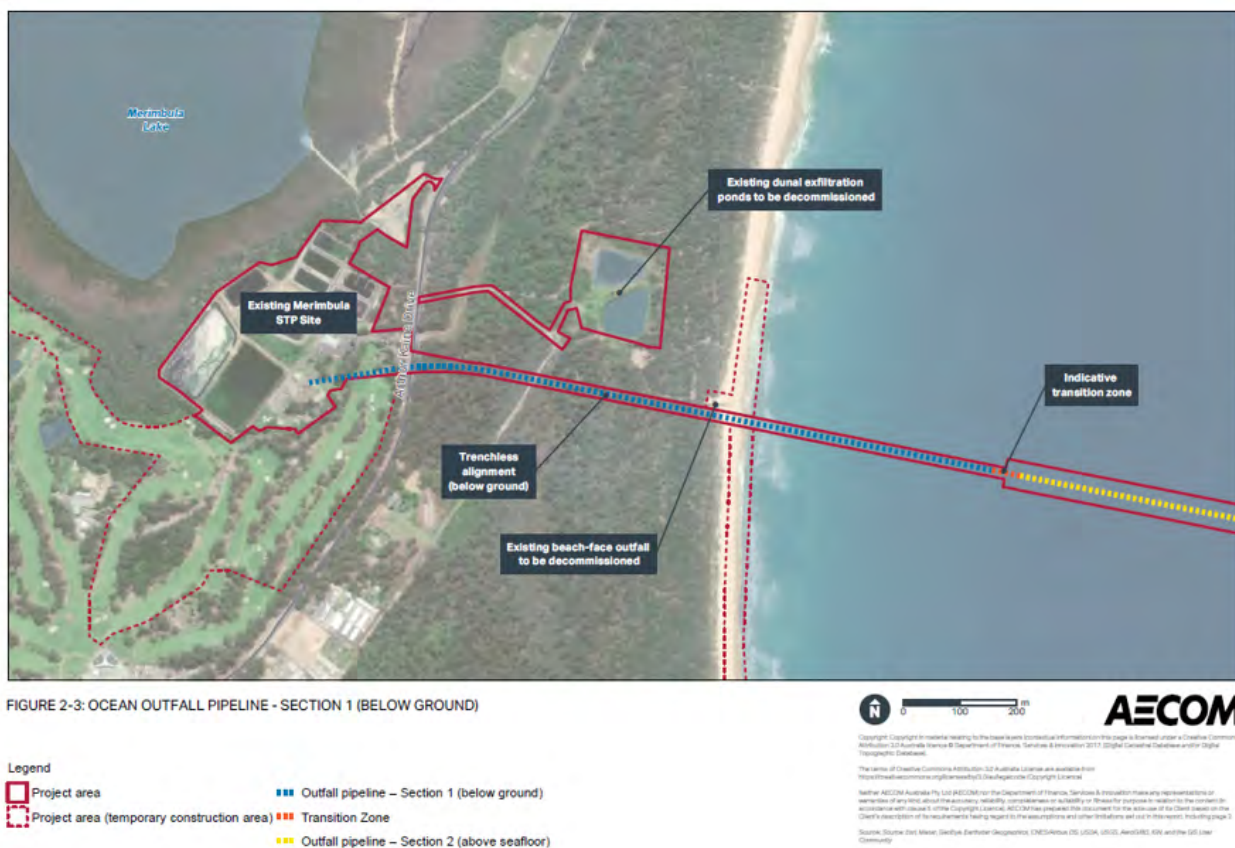
Figure 1-6 Ocean outfall pipeline – Section 1 (below ground)
