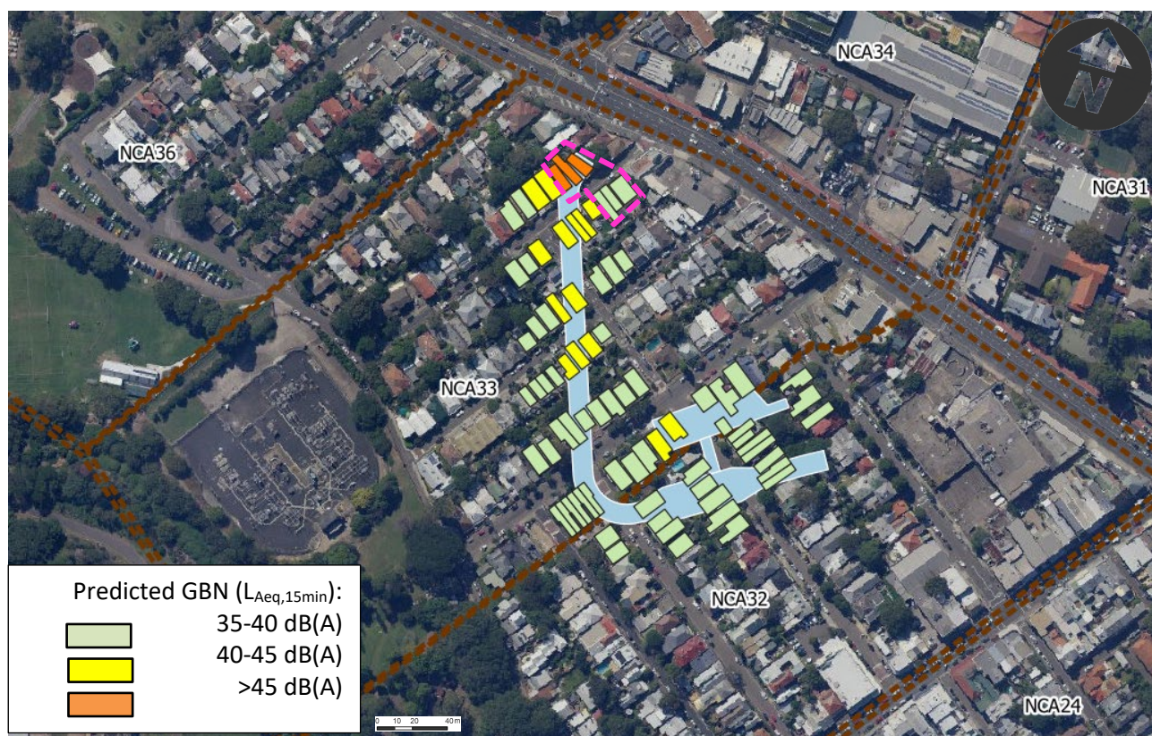
Figure 7-2 Maximum predicted GBN levels (ventilation tunnel and caverns in light blue). Properties within dashed pink area will also receive GBN from Iron Cove link tunnel excavation.
