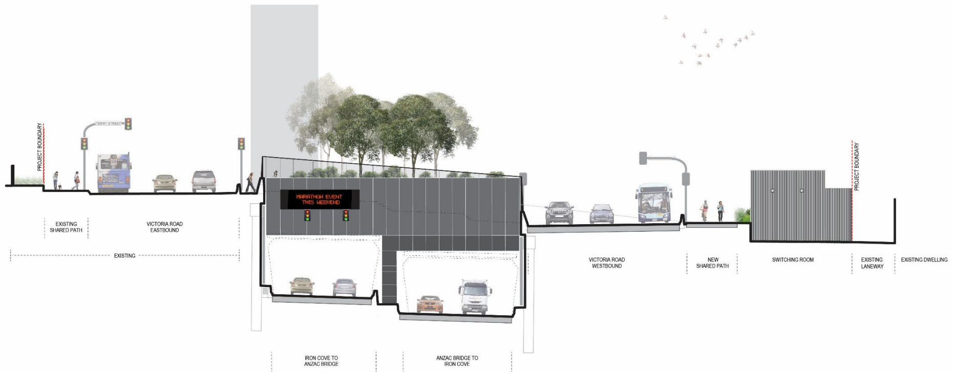
Figure 7-8 Iron Cove Link - Typical section AA
