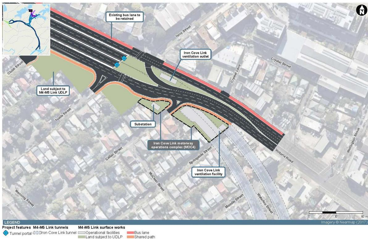
**Figure 1 EIS Location of Operational Ancillary Facilities at Iron Cove Link**
