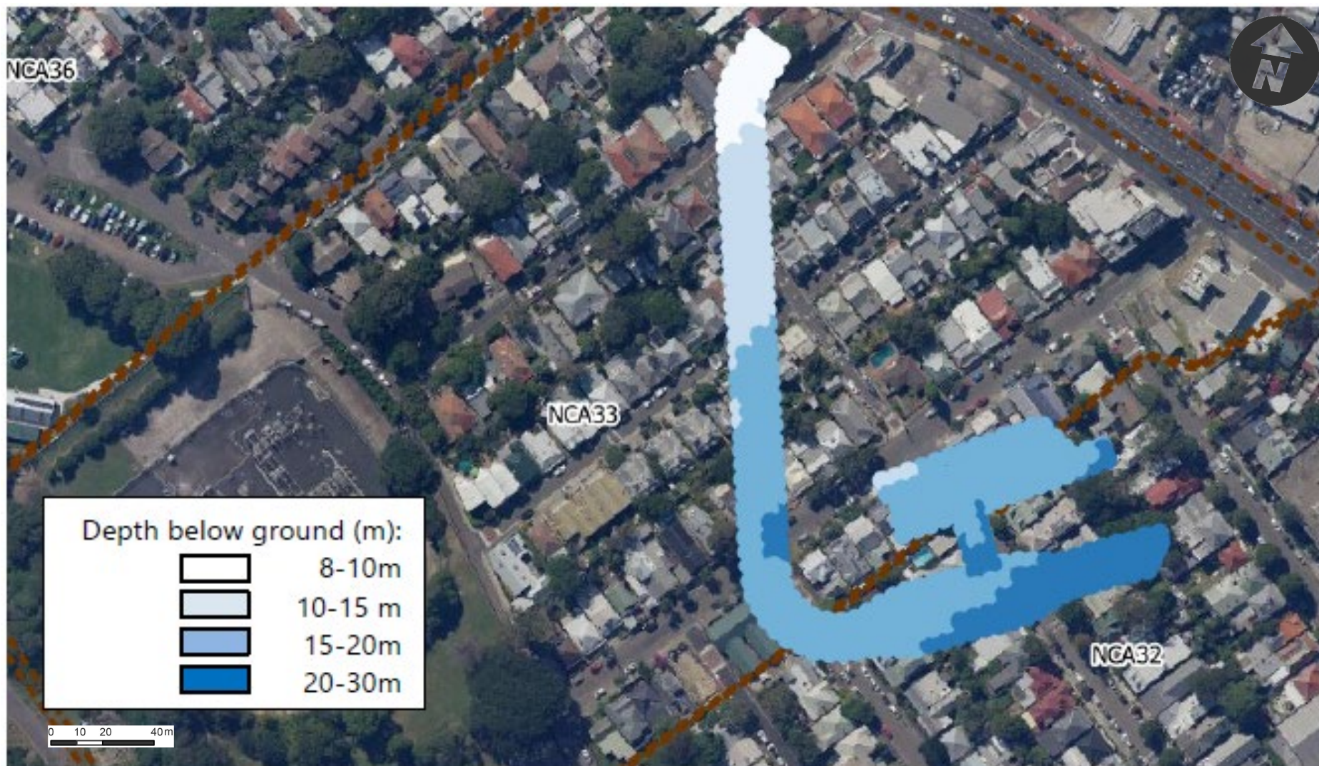
Figure 5-3 Indicative depth from ground level to crown of ventilation tunnel and caverns
