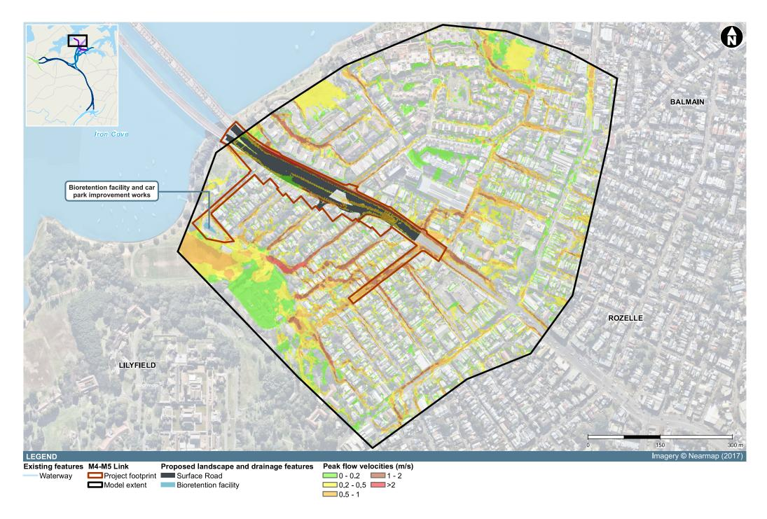
Figure 6-13 Proposed design conditions flood behaviour – Iron Cove Link - peak flow velocities (100 year ARI)
