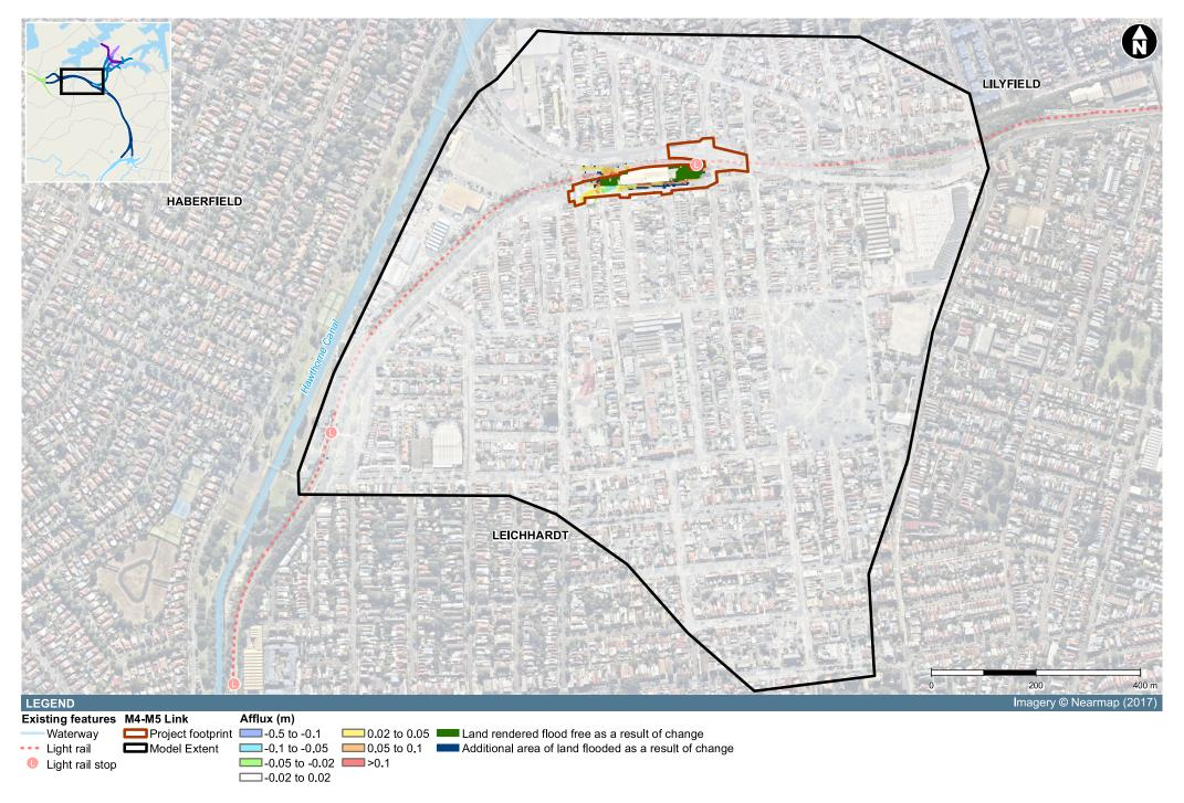
Figure 6-19 Proposed design conditions flood behaviour – Darley Road - relative flood impact (PMF)
