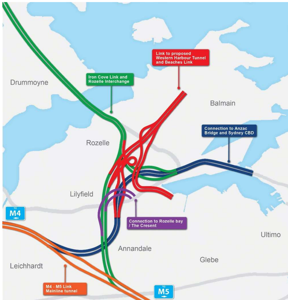
Figure 3. M4-M5 Link tunnels and roads
