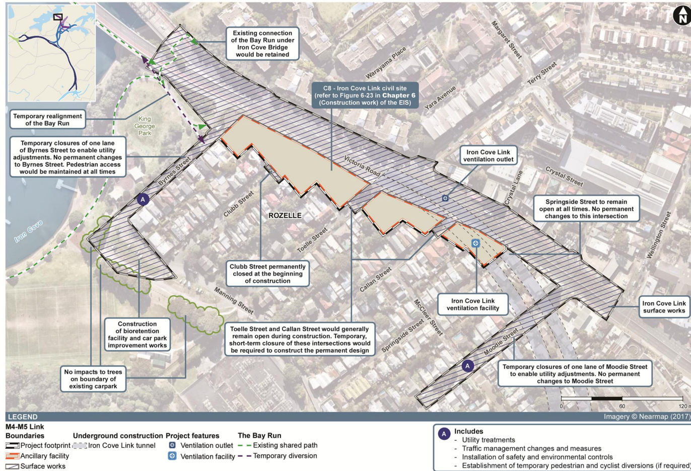
Figure 2-34 Construction ancillary facility layout at Iron Cove
