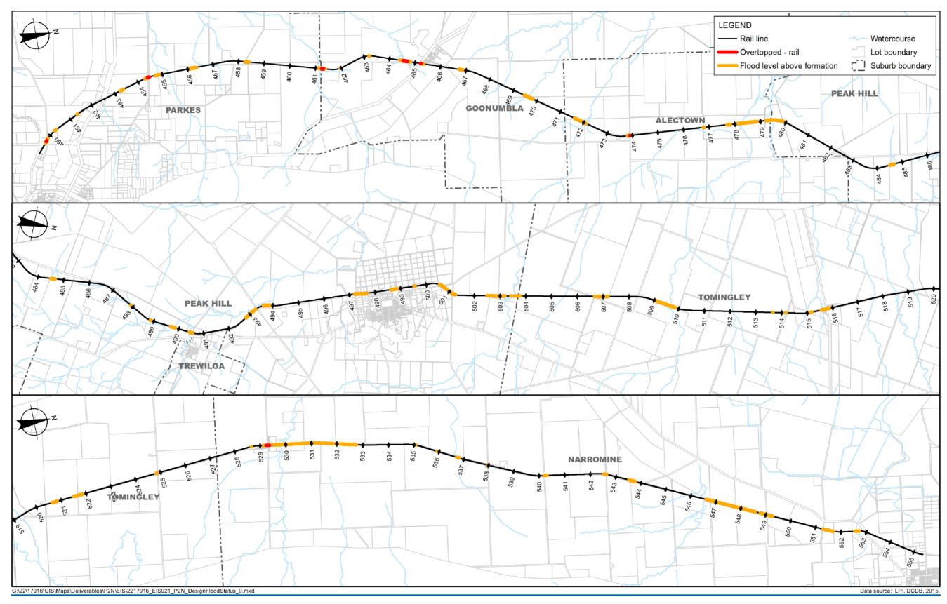
Figure 15.4 Rail overtopping during operation
