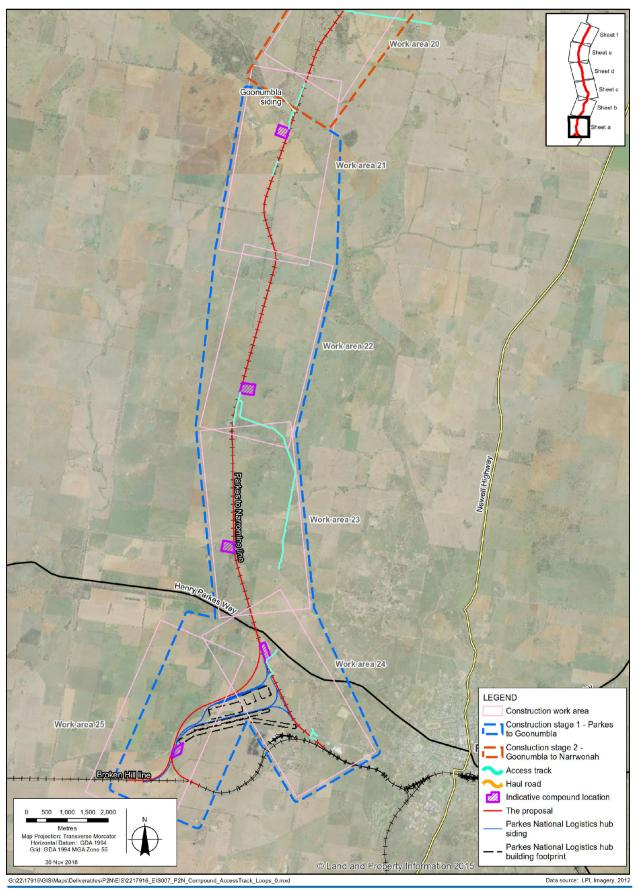
Figure 8.2a Construction work stages, work areas and compounds
