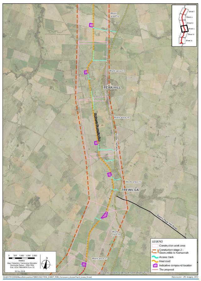
Figure 8.2c Construction work stages, work areas and compounds
