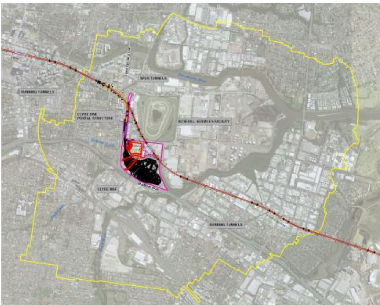
Figure 3-1. Metro West Clyde Maintenance and Stabling Facility layout, main line and TUFLOW model extent.
