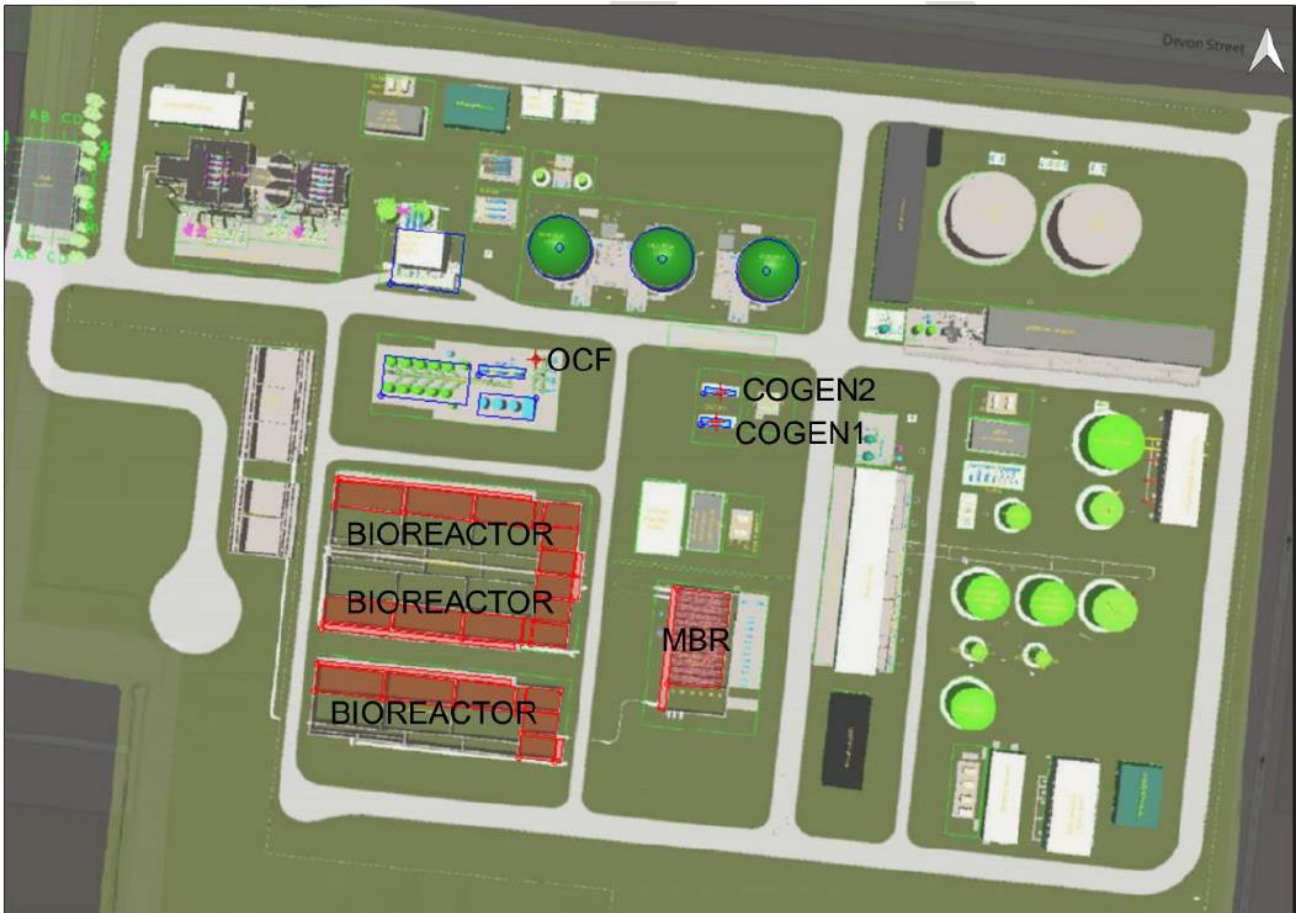
Figure 6.4: Potential emission sources used in modelling (MBR – membrane bioreactor, OCF – odour control unit, COGEN – biogas cogeneration unit)
