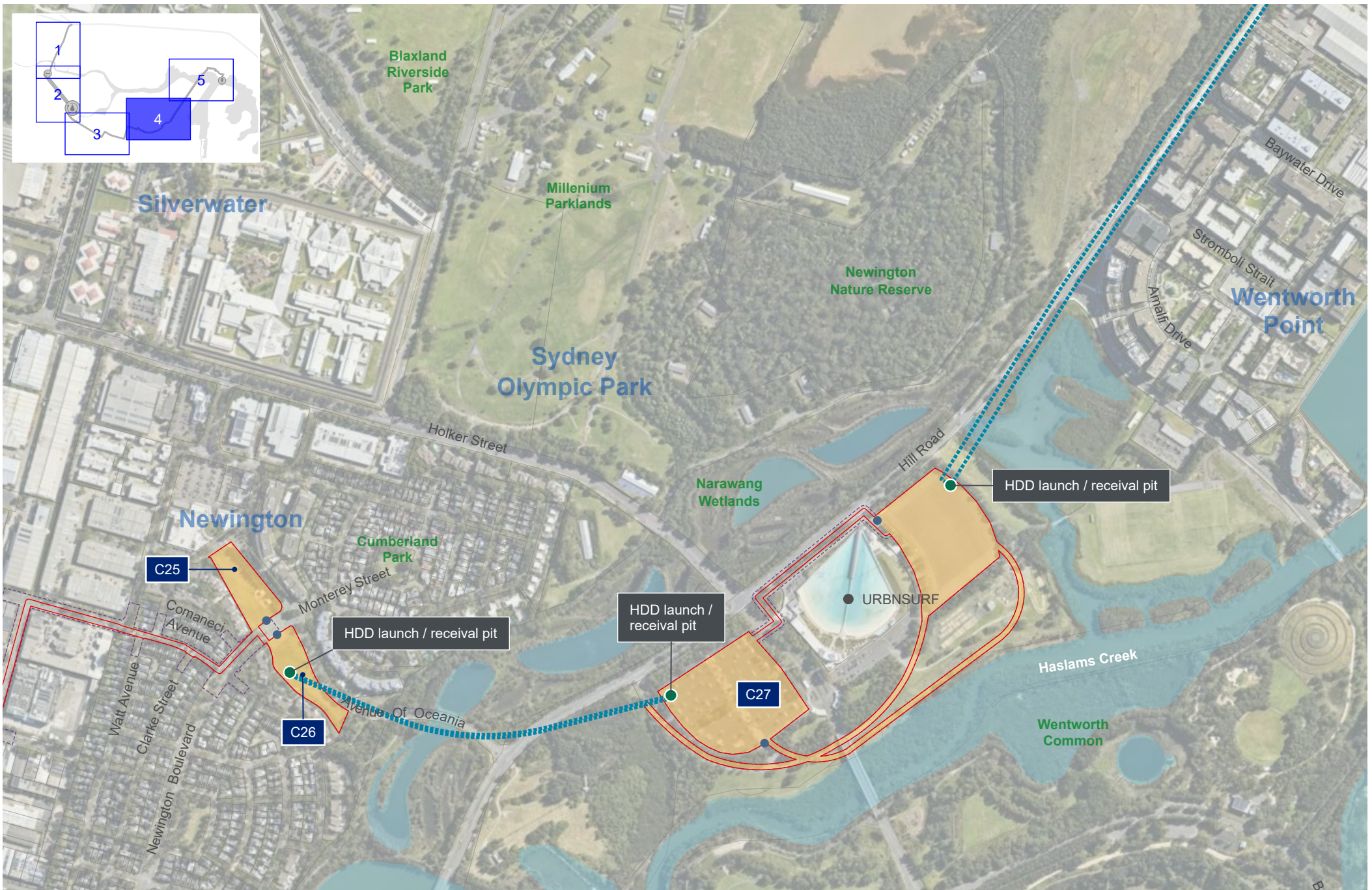
Figure B-4 Project impact area including indicative construction compounds
