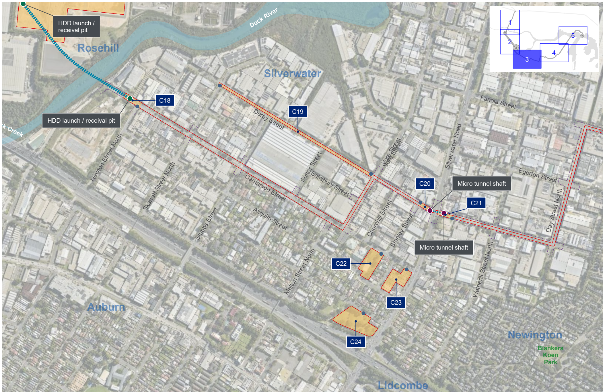
Figure B-3 Project impact area including indicative construction compounds
