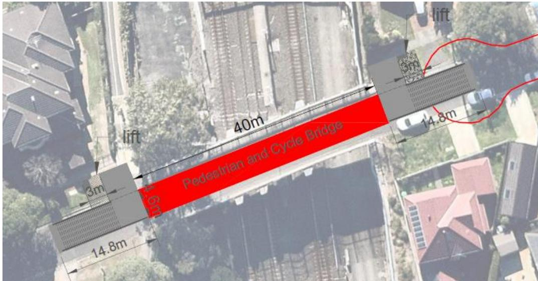
Figure 27: Nelson Street Stairs and Lift option – footprint
