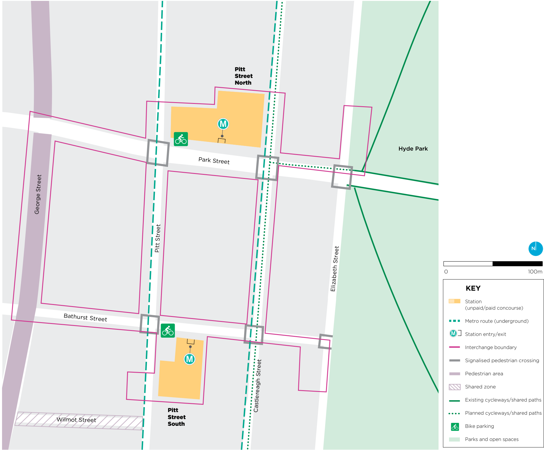
Pitt Street Station – cycling interchange and transfer requirements
