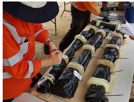
Timbers being fastened to board with brackets shaped individually to help preserve the curve of each timber. Source: Irini Malliaros/Silentworld Foundation
