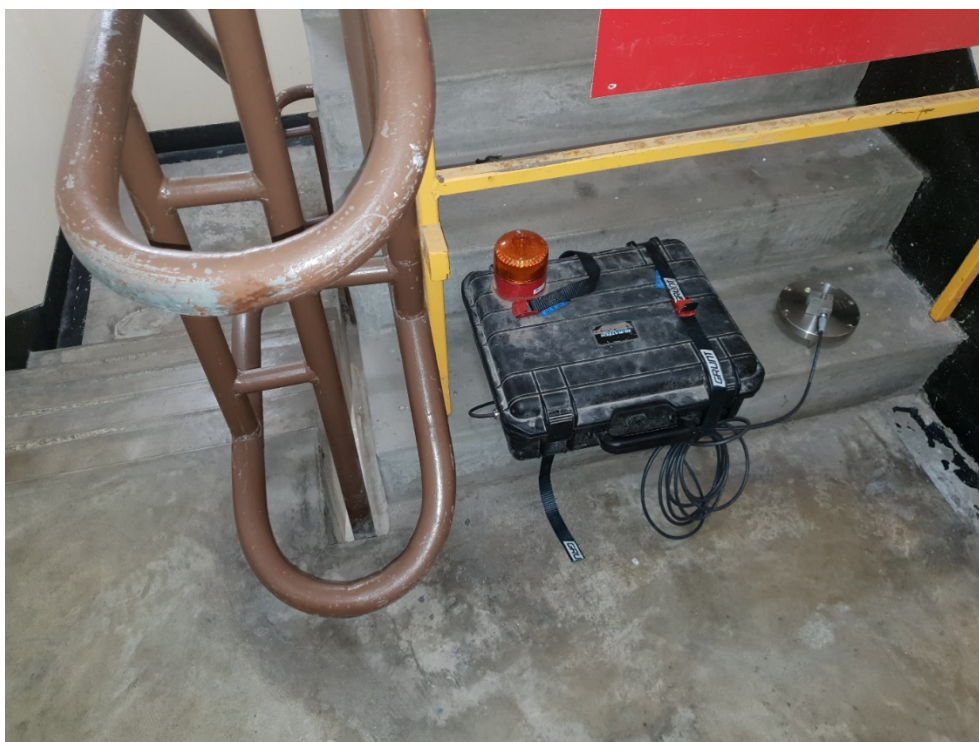
Figure 2-2: Unattended vibration Logger set up at the Dental Hospital southern stairwell
