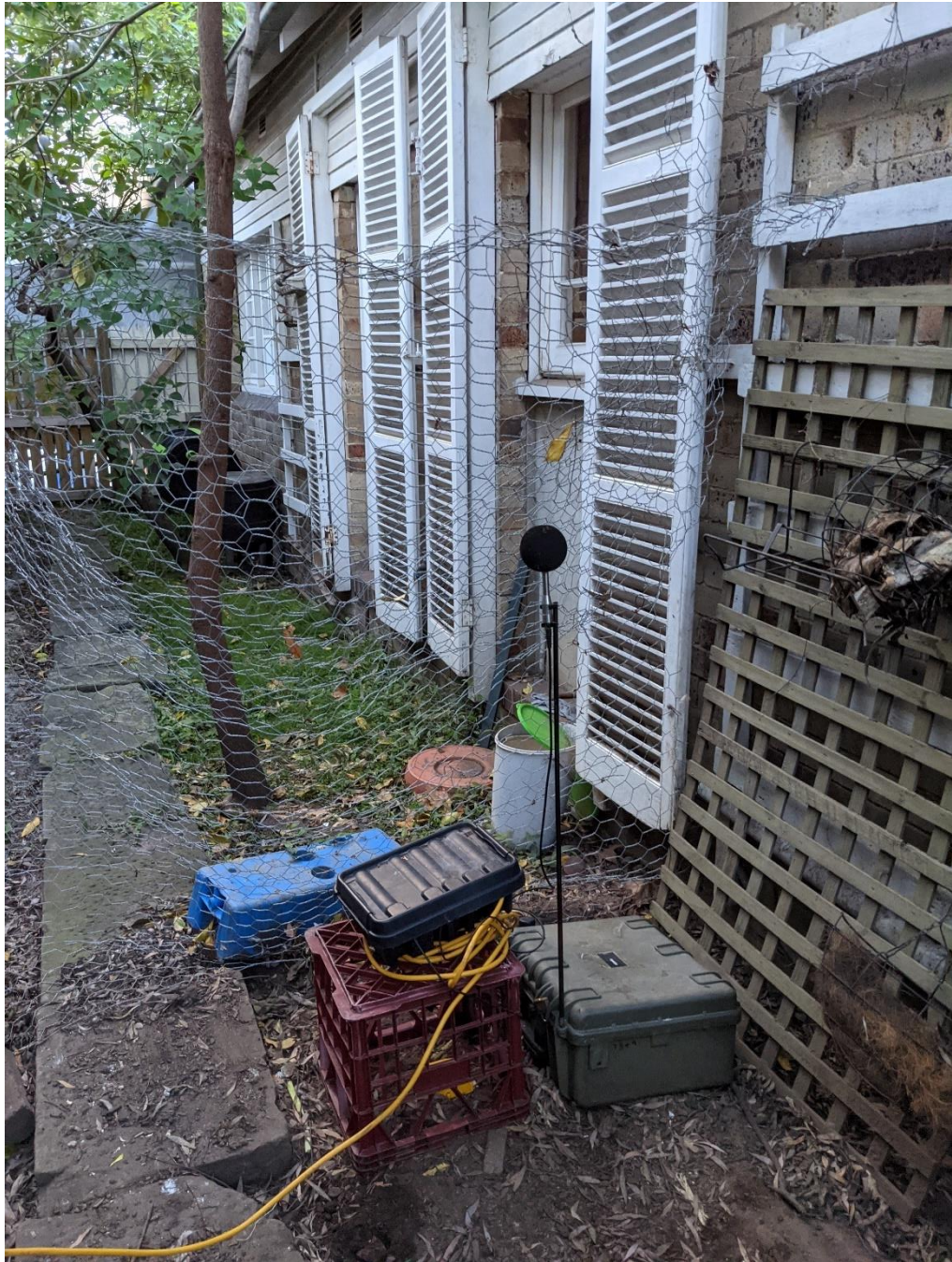
Figure 10 Real-time Noise and Vibration Monitors at 243 Miller Berry St eastern boundary (after relocation on 27 May 2021)
