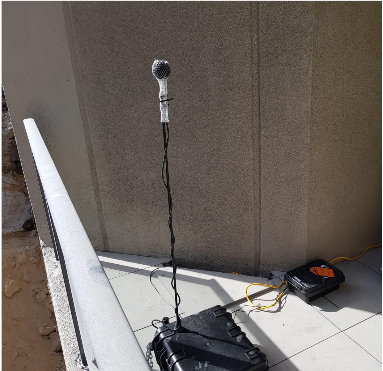
Figure 8 Real-time Noise and Vibration Monitors at 65 Berry St Ground floor balcony
