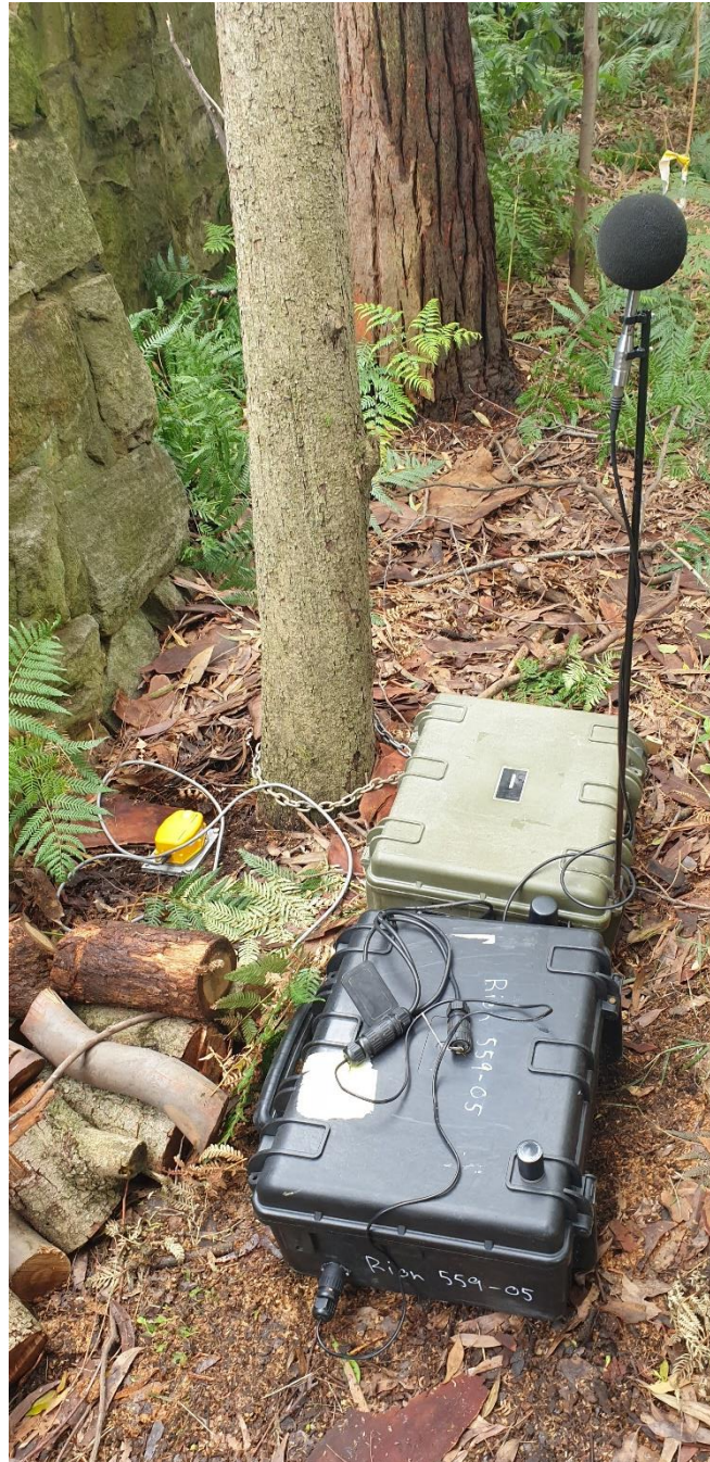
Figure 9 Real-time Noise and Vibration Monitors at 243 Miller Berry St southern boundary (before relocation on 27 May 2021)
