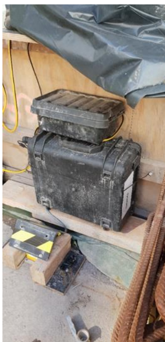
Figure 2-5b: Real time vibration logger 30 Chalmers St relocated to centre of site January 2021)
