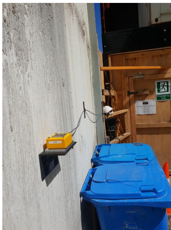
Figure 2-5a: Real time vibration logger setup on the wall of 30 Chalmers St (installed 14 October 2019- January 2021)
