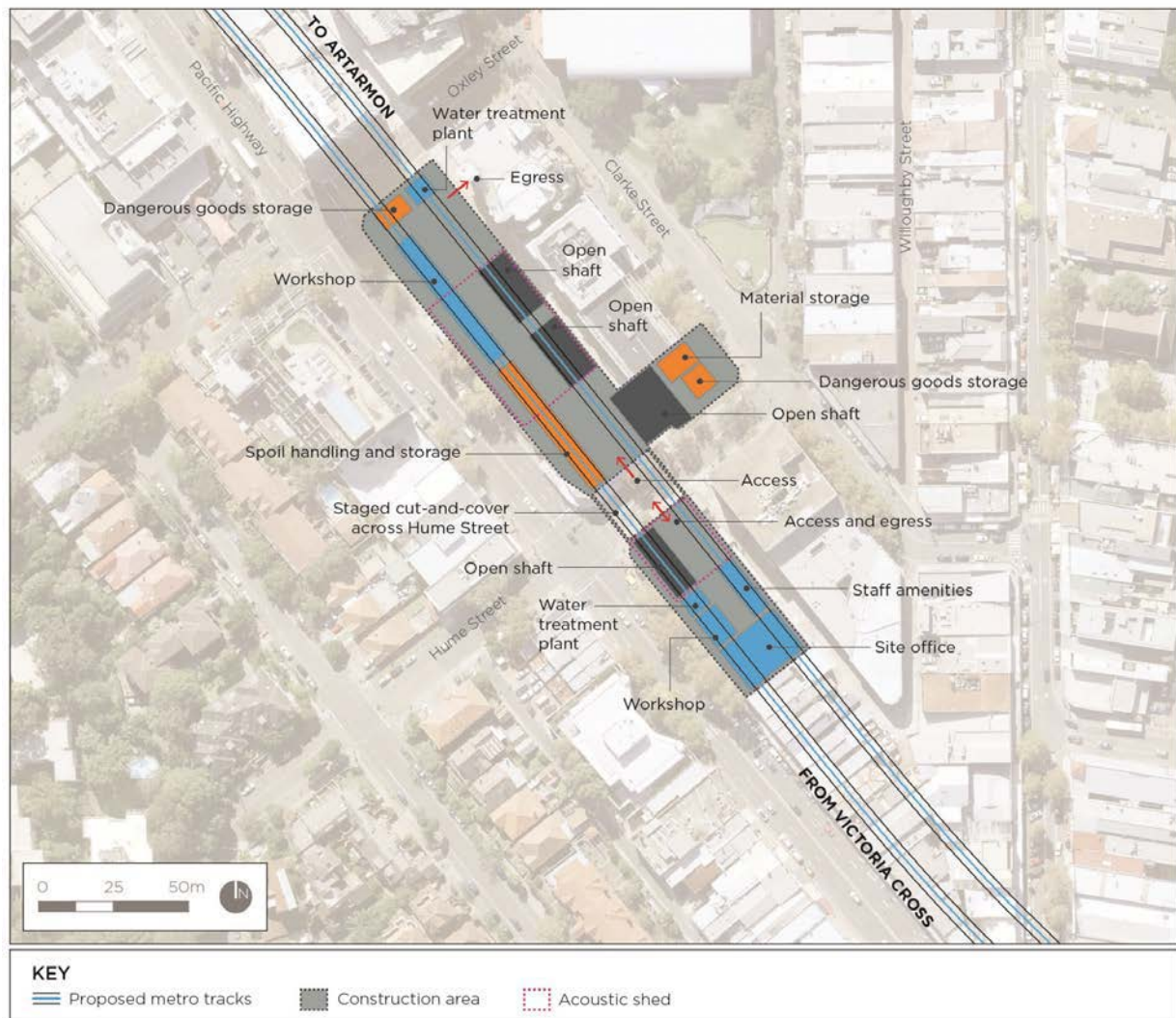
Figure 30: Crows Nest Station construction site layout.
