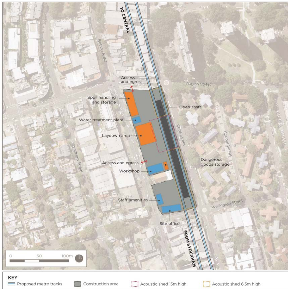
Figure 178: Waterloo Station construction site layout
