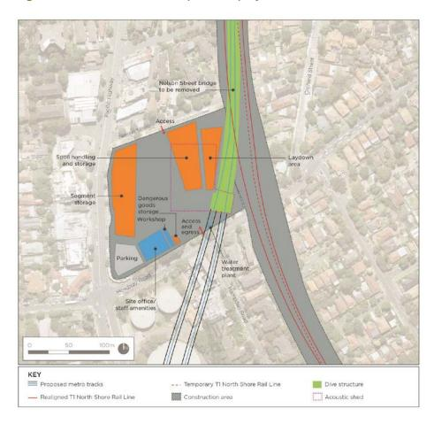
The southern portion of the site would be used for offices, workshops and car parking; spoil storage and handling would be located at the northern end of the site adjacent to the existing rail line, with segment storage adjacent to the Pacific Highway. The dive structure would be constructed in the eastern portion of the site. The location and indicative layout of the Chatswood dive site, including vehicle access / egress is illustrated in Figure 4.
