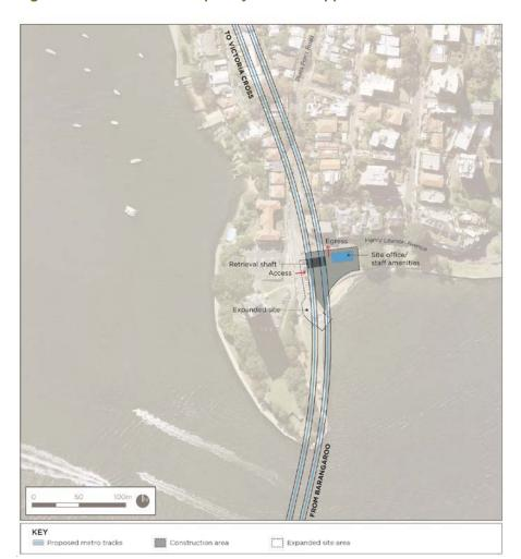
Figure 66: Blues Point Temporary Tunnel Support Site.
