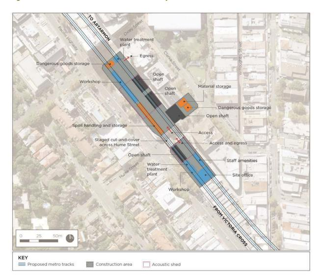
Figure 30: Crows Nest Station construction site layout.
