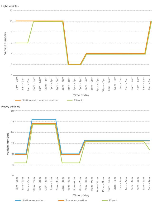
Figure 3-3 Barangaroo track cross-over - hourly traffic profile of construction vehicles (arrival only)
