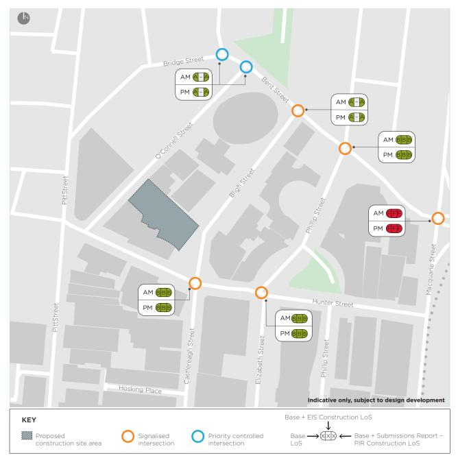
Figure 3-14 Martin Place Station construction sites plus the O'Connell Street site
