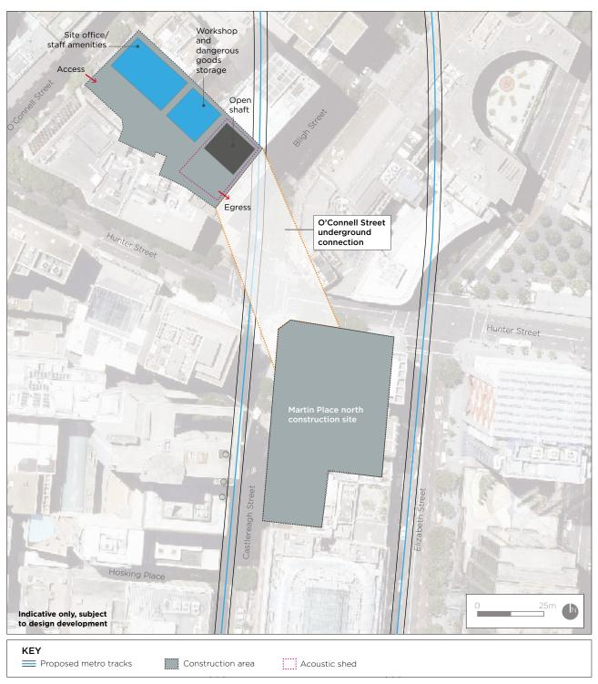
Figure 3-11 O'Connell Street - indicative construction site layout
