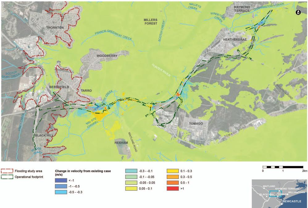
Figure 10-35 Change in flow velocity during operation (1% AEP)
