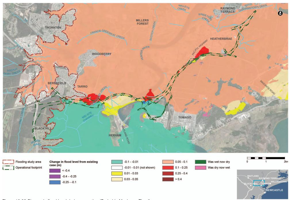
Figure 10-32 Change in flood level during operation (Probable Maximum Flood) Expendence Extension Structure Topology Structure
