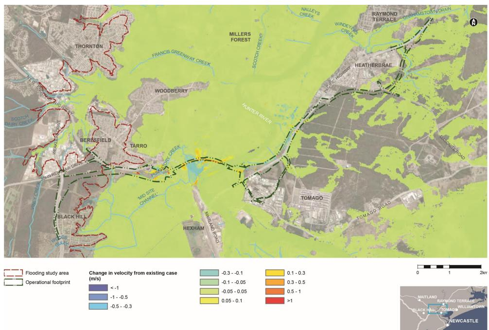
Figure 10-34 Change in flow velocity during operation (5% AEP)
