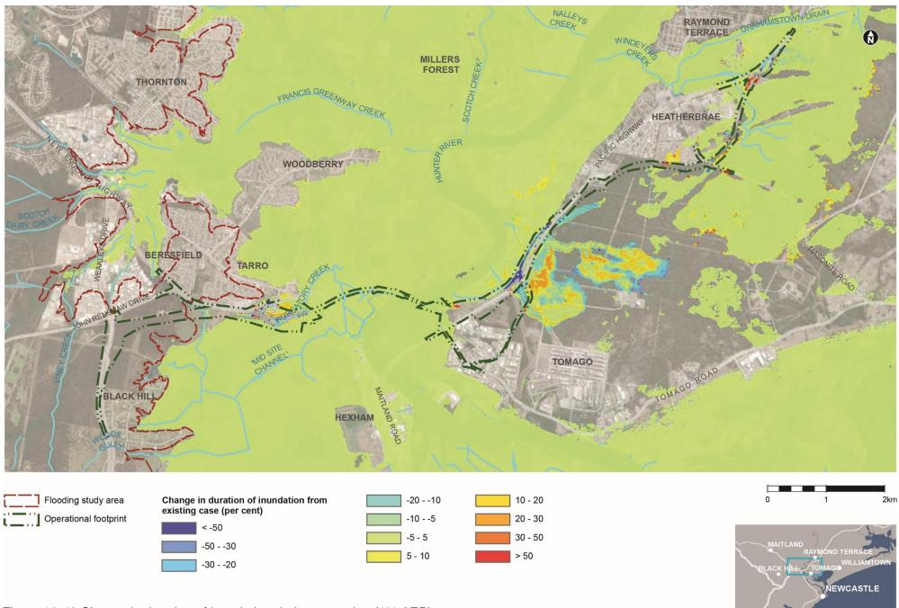
Figure 10-43 Change in duration of inundation during operation (1% AEP)
