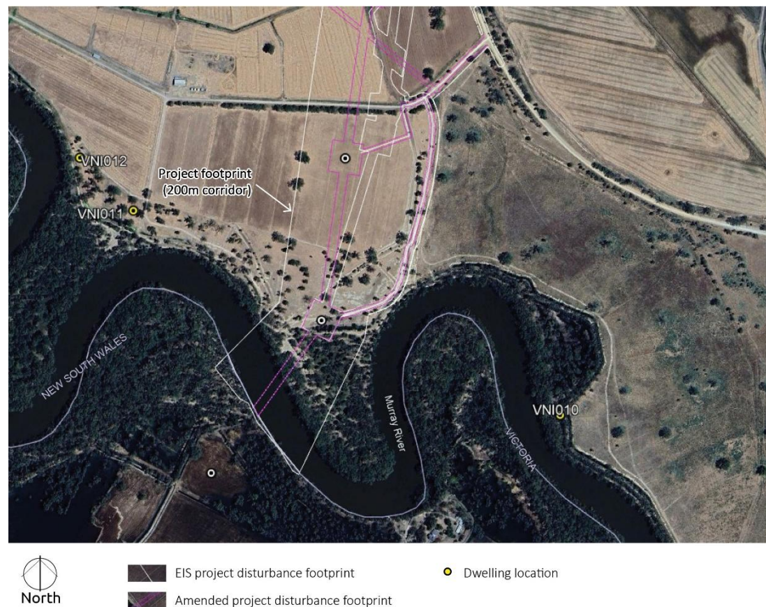
FIGURE 4-1 AMENDED PROJECT FOOTPRINT AND INDICATIVE DISTURBANCE FOOTPRINT IN THE VICINITY OF VNI010
