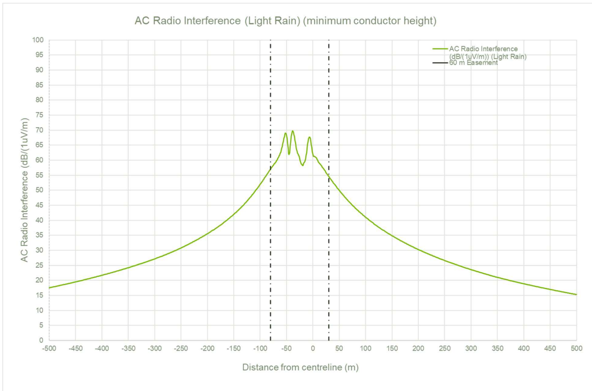
Figure 6-5: Scenario 2 AC Radio Interference (L50) minimum conductor height
