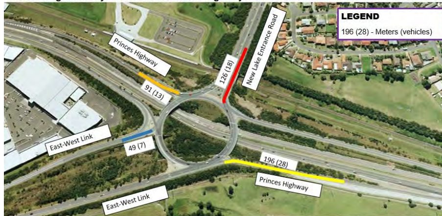
Queue Length Surveyed in 2014 at Princes Highway/East West Link/New Lake Entrance Road intersection 4.00-4.15 PM
