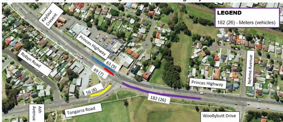
Queue Length Surveyed in 2014 at Tongarra Road/Princes Highway intersection 8.30-8.45AM
