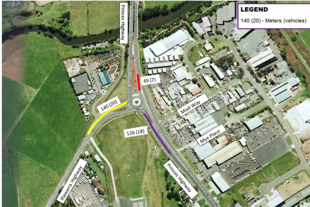
Figure 4-14 Existing AM Peak Queue Length at Princes Highway and Illawarra Highway Intersection
