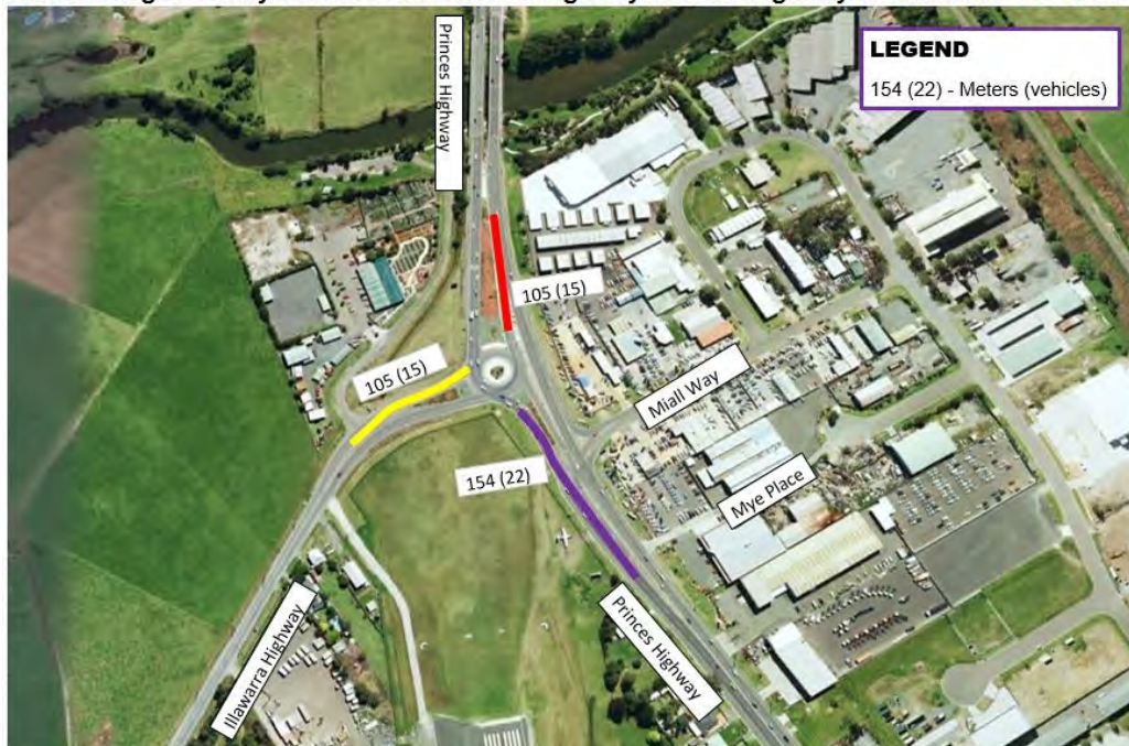
Figure 4-15 Existing PM Peak Queue Length at Princes Highway and Illawarra Highway Intersection
