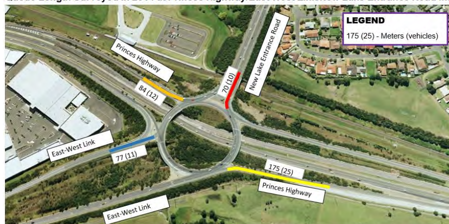
Figure 4-20 Existing AM Peak Queue Length at the Oak Flats Interchange
