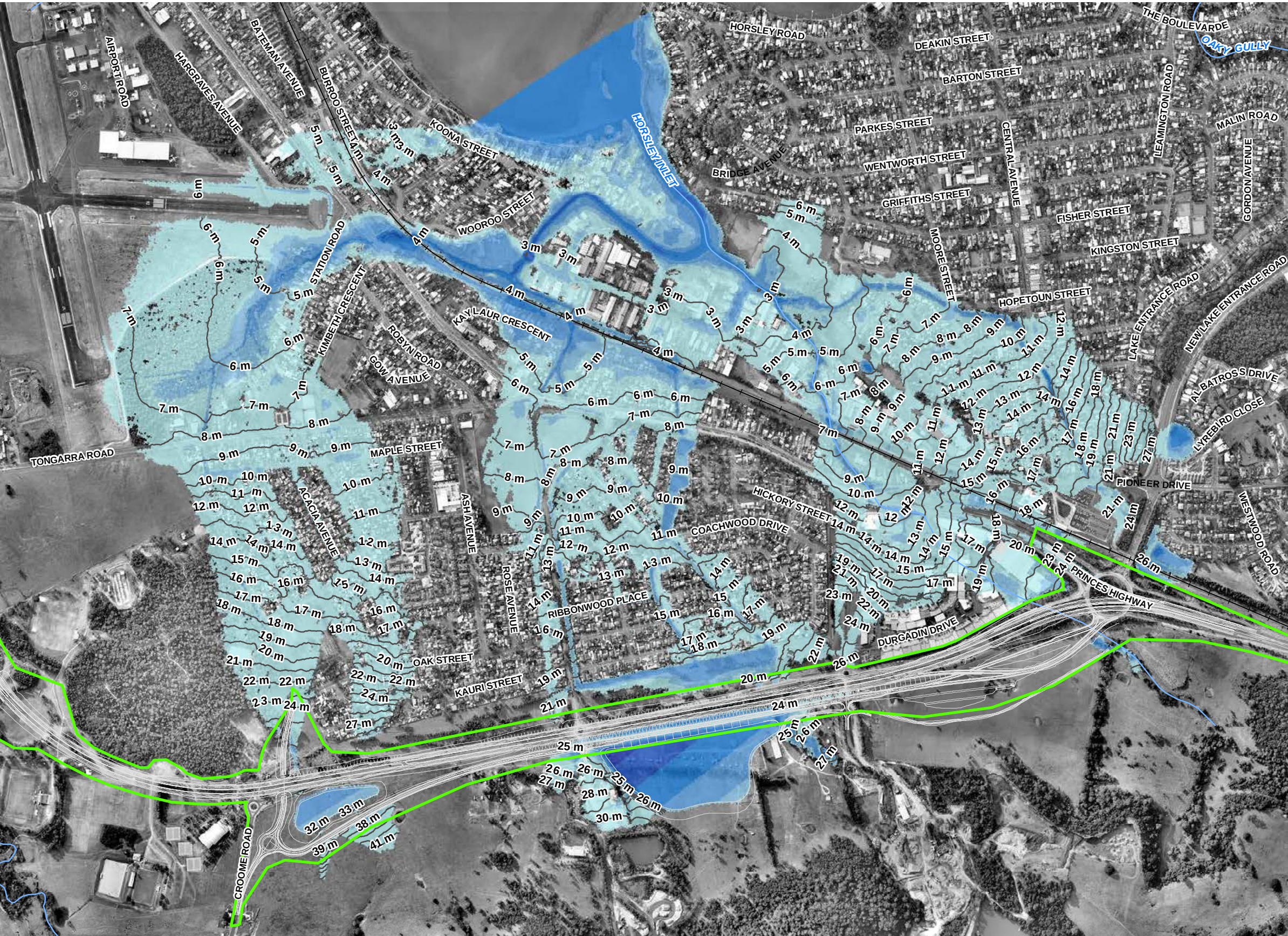
HORSLEY CREEK 100 YEAR ARI FLOOD DEPTH – WITH PROPOSED BYPASS
