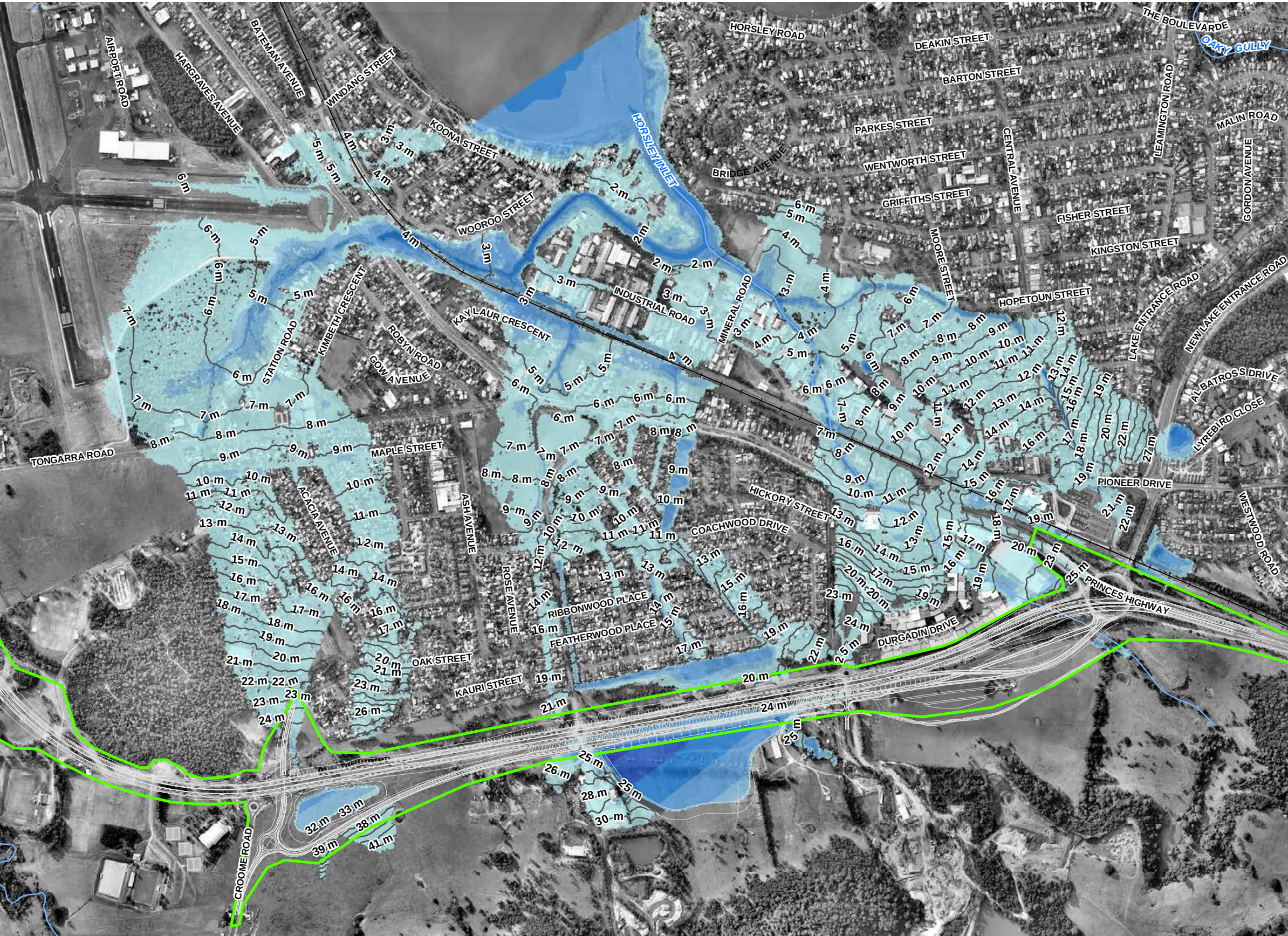
HORSLEY CREEK 20 YEAR ARI FLOOD DEPTH – WITH PROPOSED BYPASS
