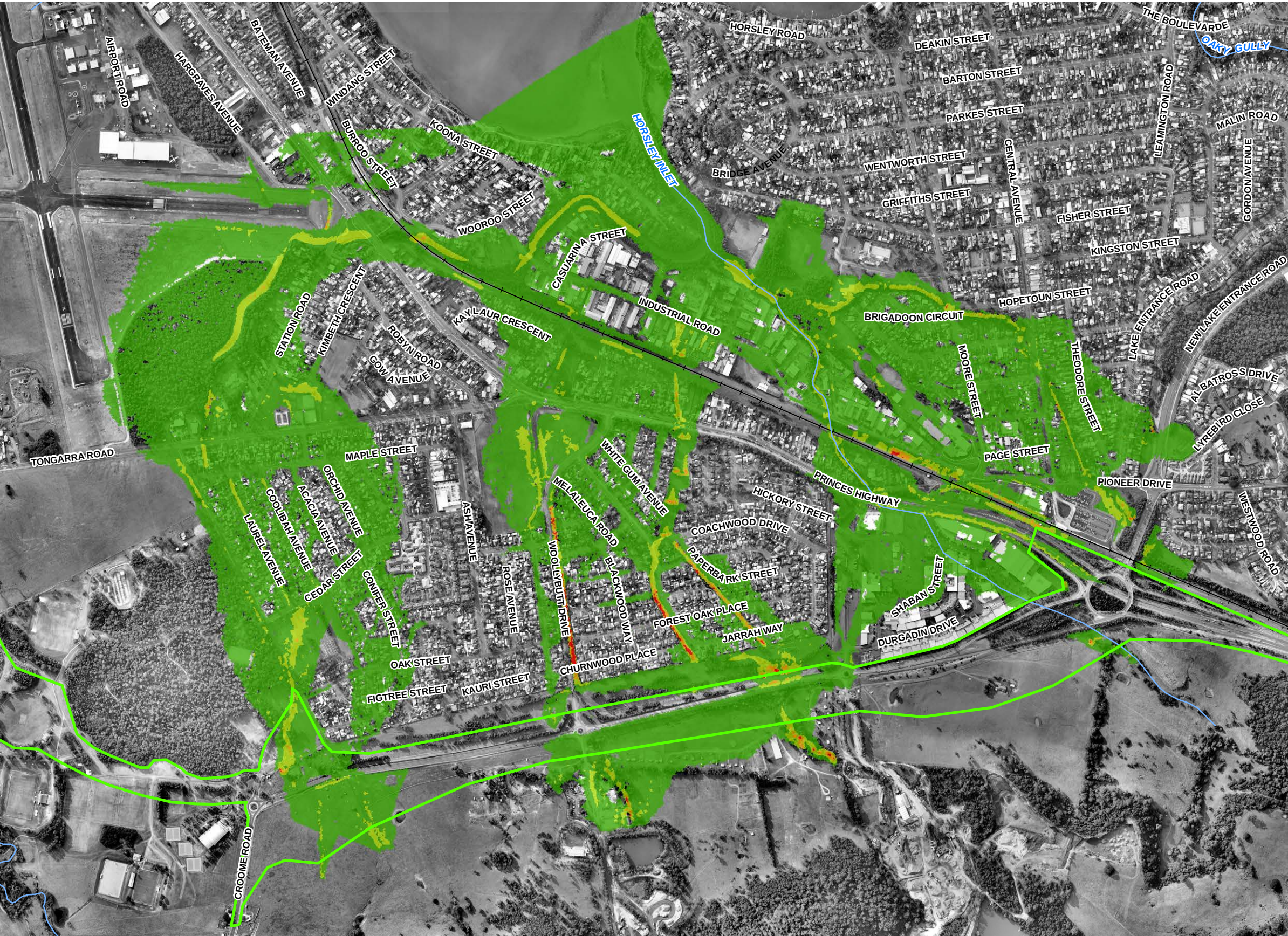
HORSLEY CREEK 100 YEAR ARI FLOOD VELOCITY – EXISTING CONDITIONS
