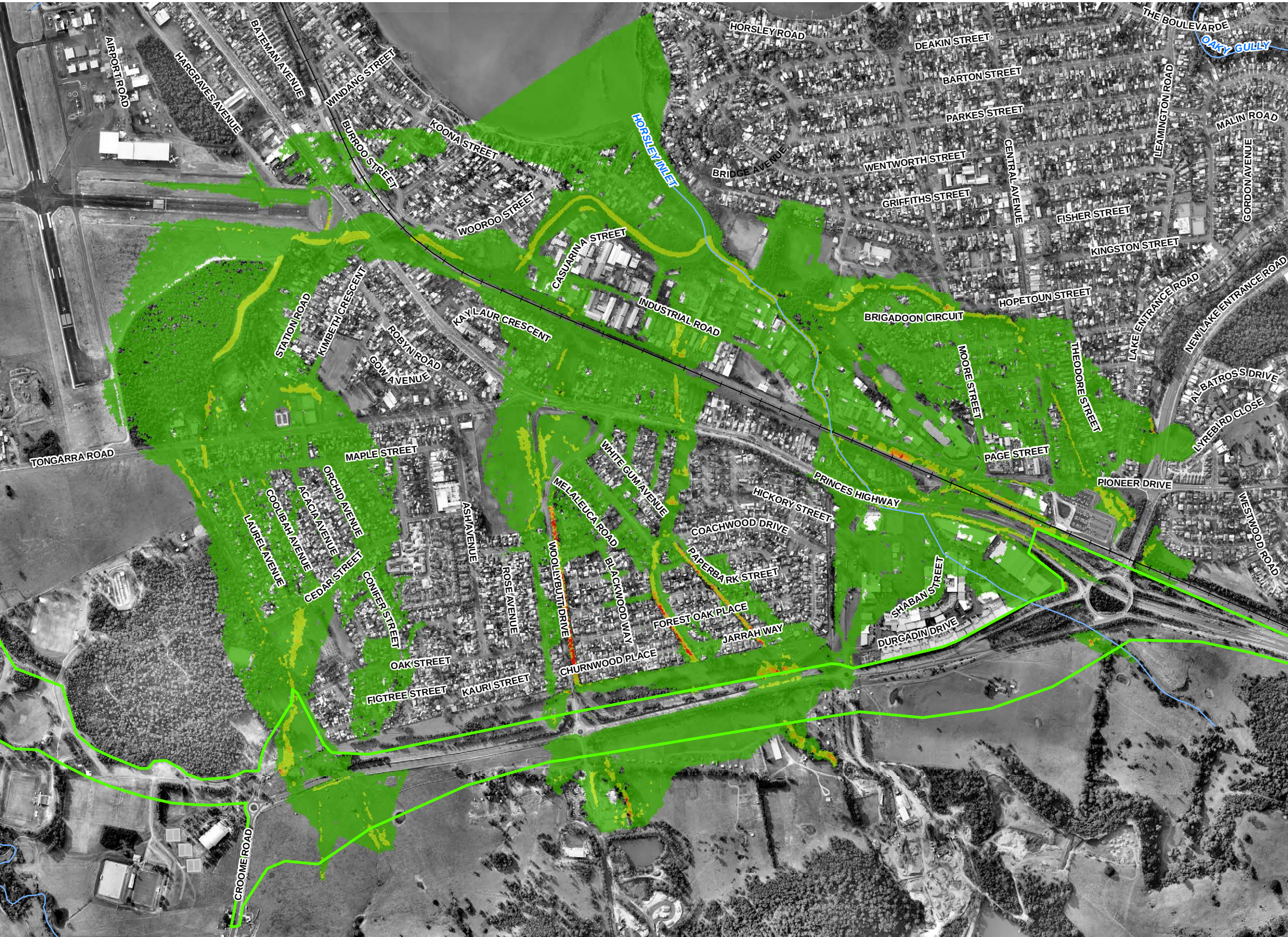
HORSLEY CREEK 50 YEAR ARI FLOOD VELOCITY – EXISTING CONDITIONS
