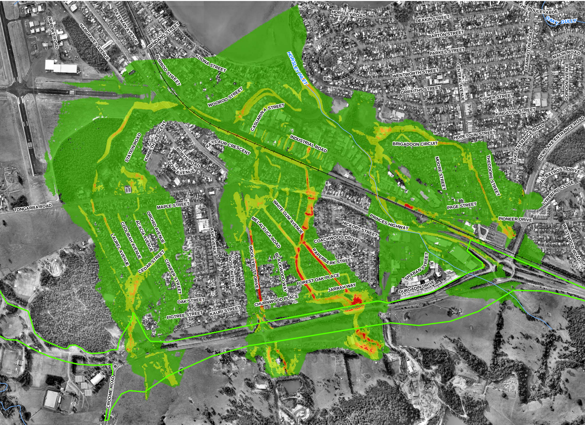
HORSLEY CREEK PMF FLOOD VELOCITY - EXISTING CONDITIONS
