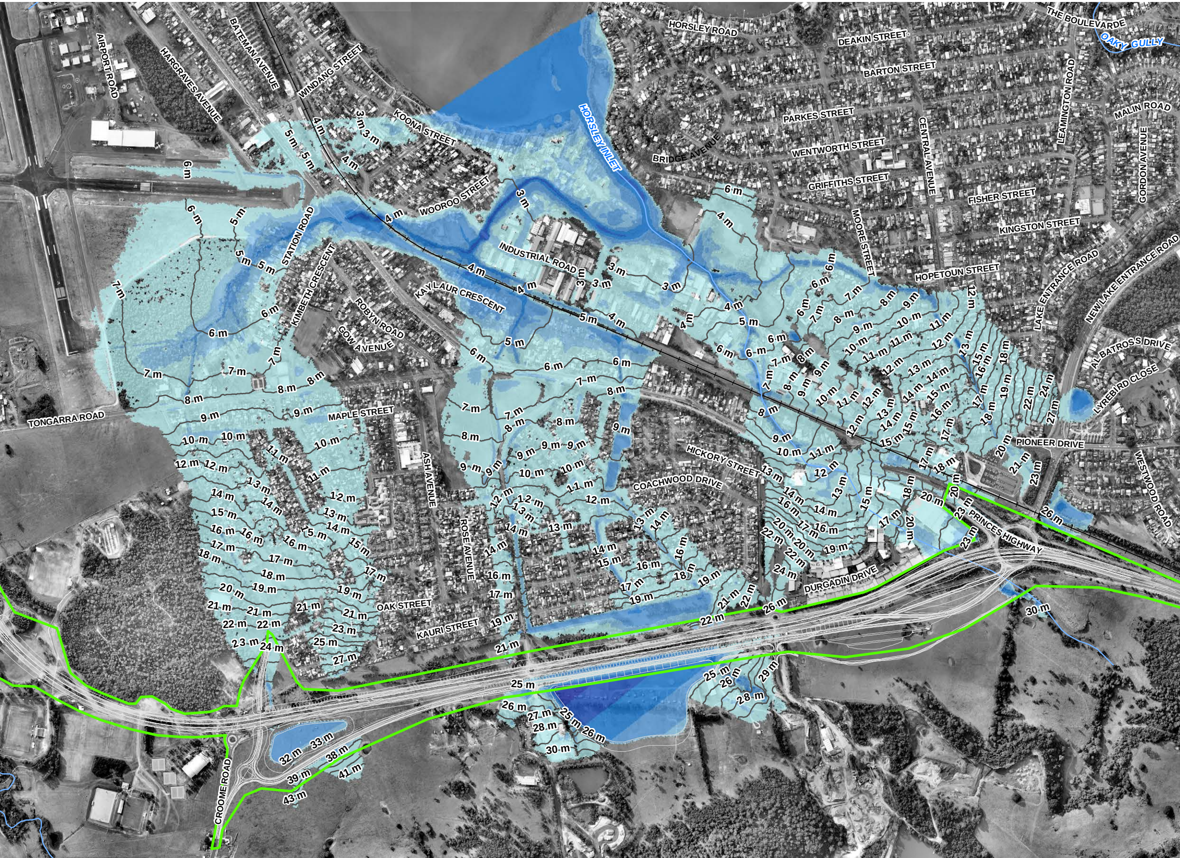
HORSLEY CREEK 200 YEAR ARI FLOOD DEPTH – WITH PROPOSED BYPASS
