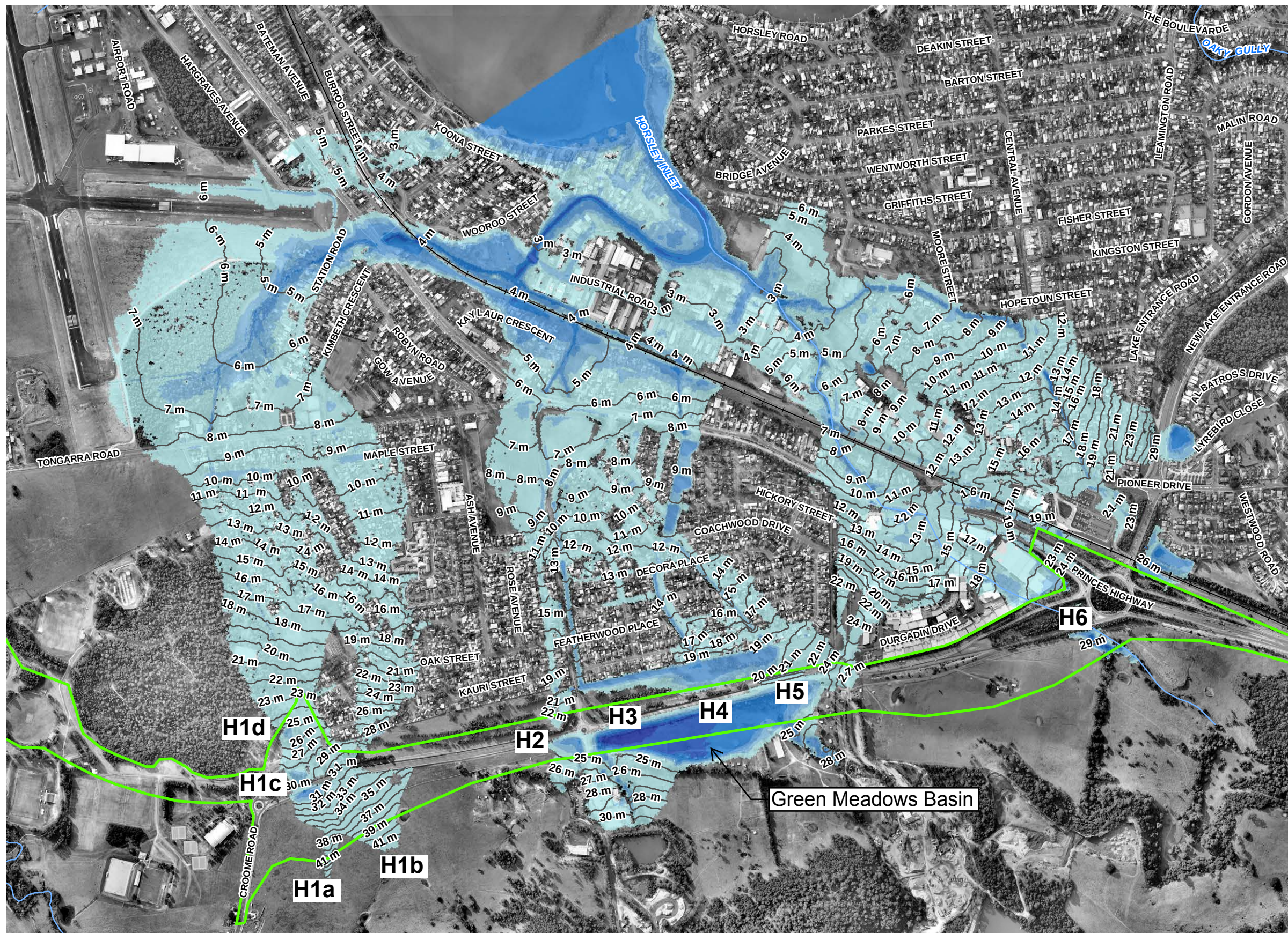
HORSLEY CREEK 100 YEAR ARI FLOOD DEPTH – EXISTING CONDITIONS
