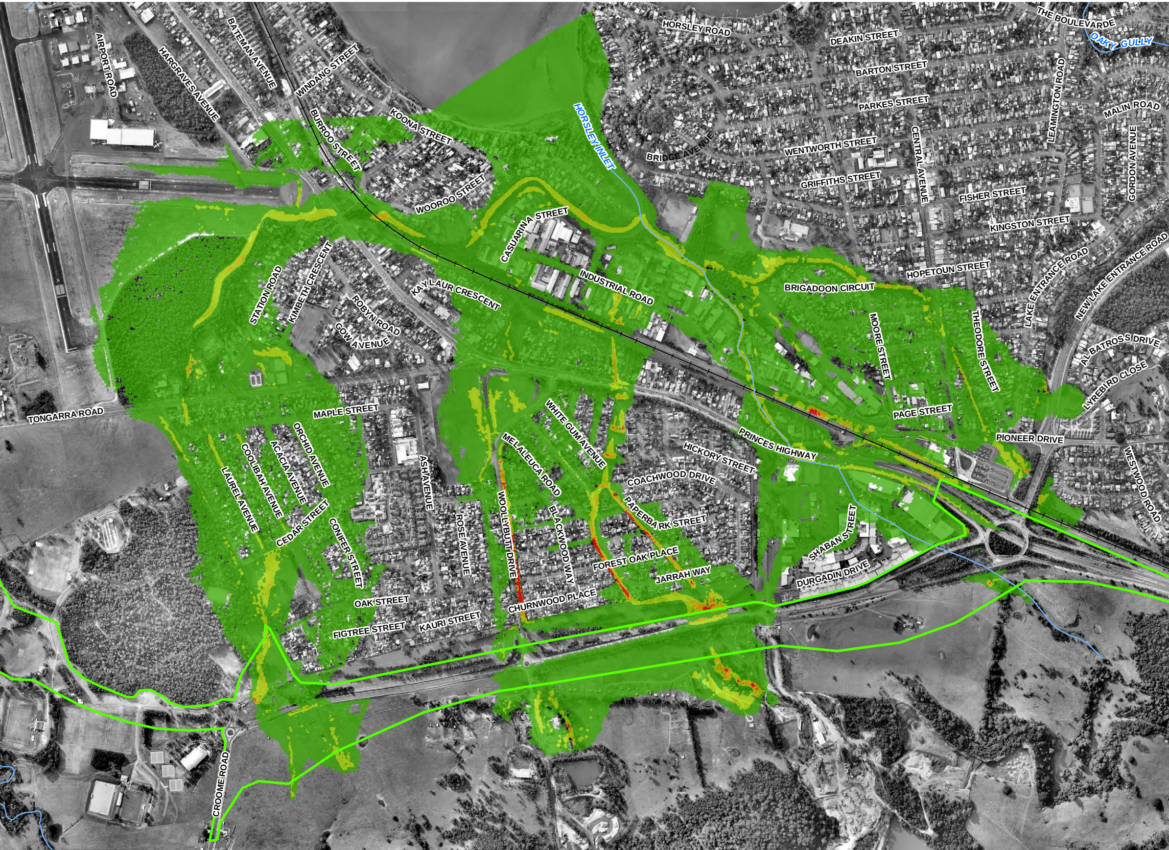
HORSLEY CREEK 200 YEAR ARI FLOOD VELOCITY – EXISTING CONDITIONS
