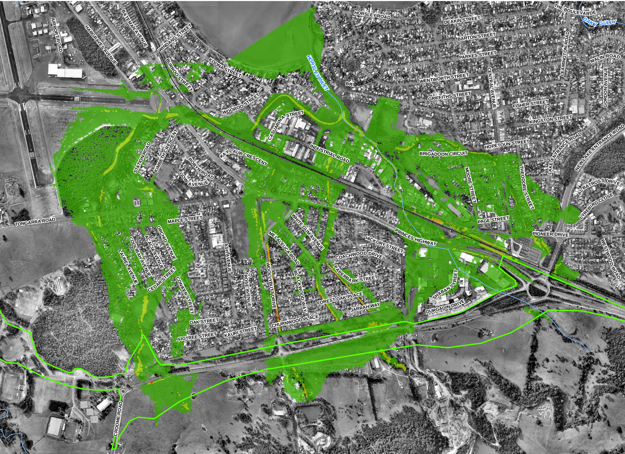
HORSLEY CREEK 10 YEAR ARI FLOOD VELOCITY – EXISTING CONDITIONS
