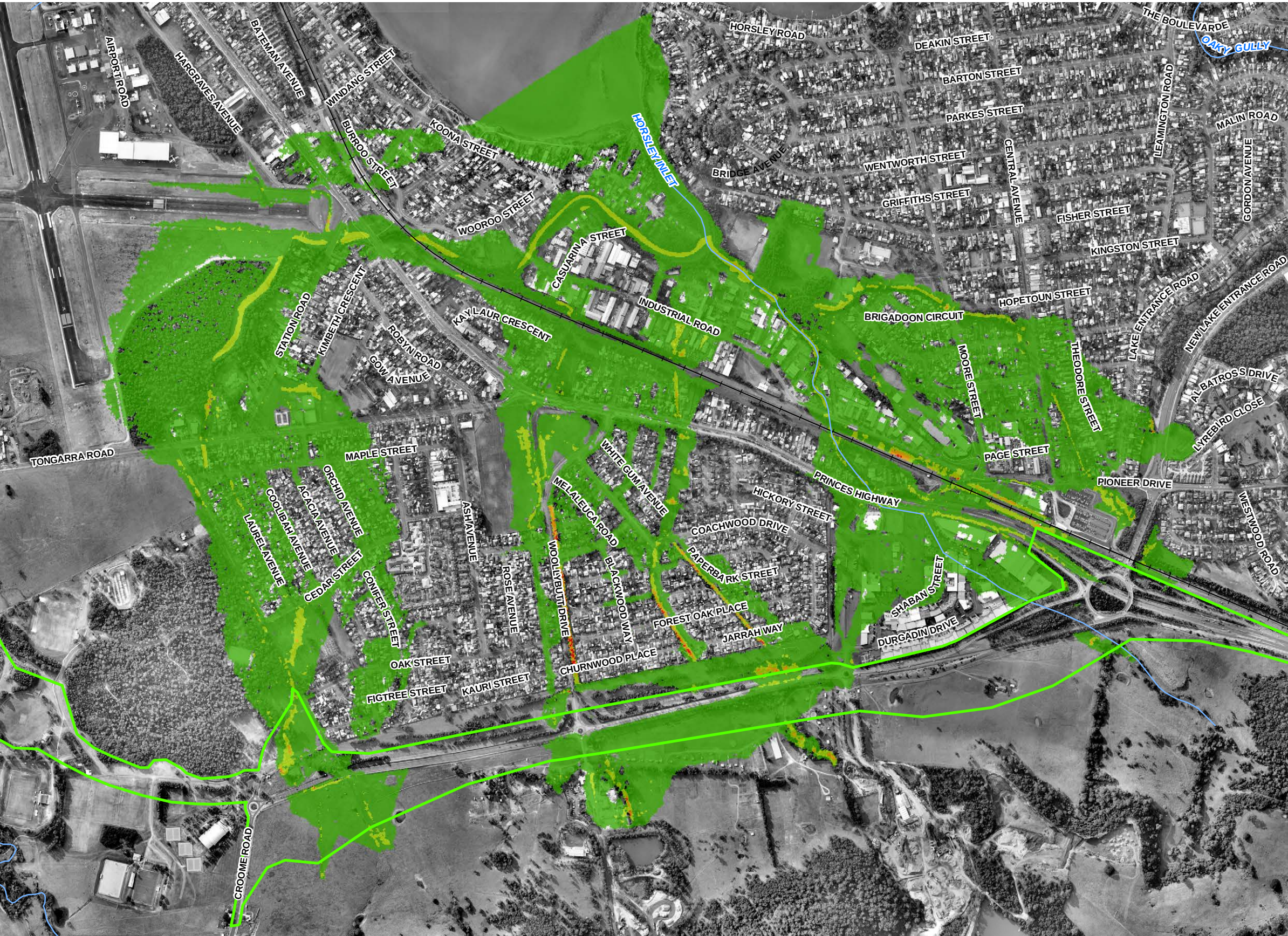
HORSLEY CREEK 20 YEAR ARI FLOOD VELOCITY – EXISTING CONDITIONS
