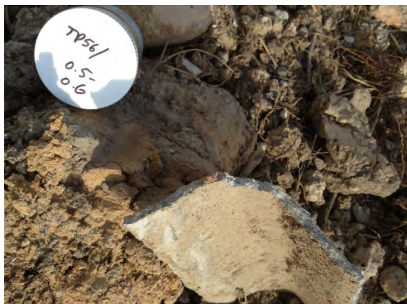
Photo 7 – ACM encountered in vicinity of TP56. Asbestos section of the site cordoned off
