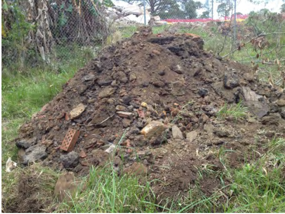
Photo 13 – Spoil excavated from TP62 showing C&D waste
