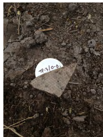
Photo 4 – ACM on ground in vicinity of TP13
