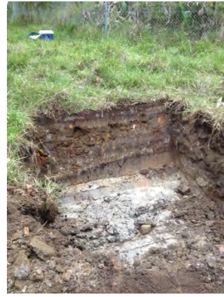
Photo 14 – Rubble fill layer in TP62 to 1.0m bgl
