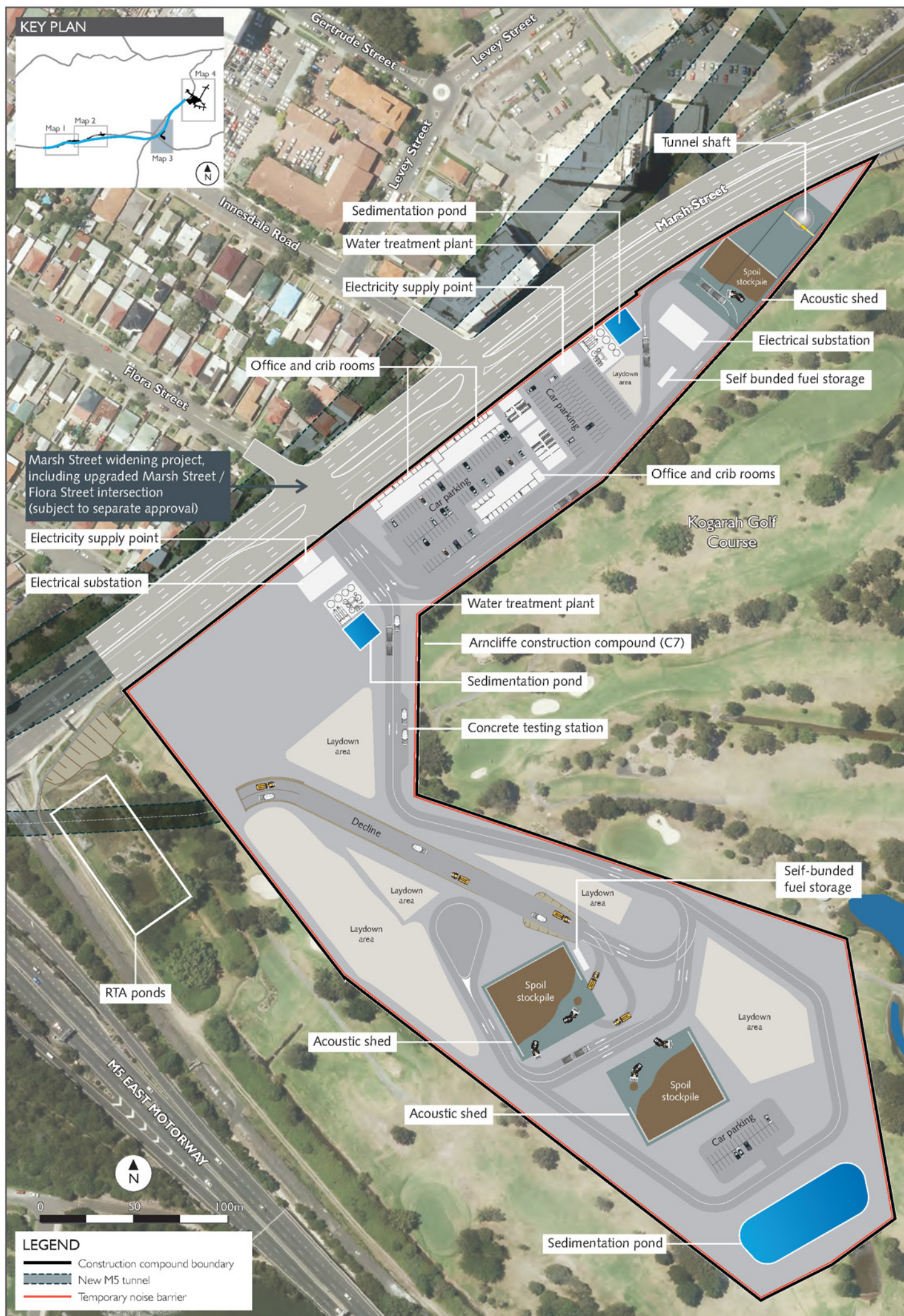
Figure 6-3 Project construction footprint - map 3
