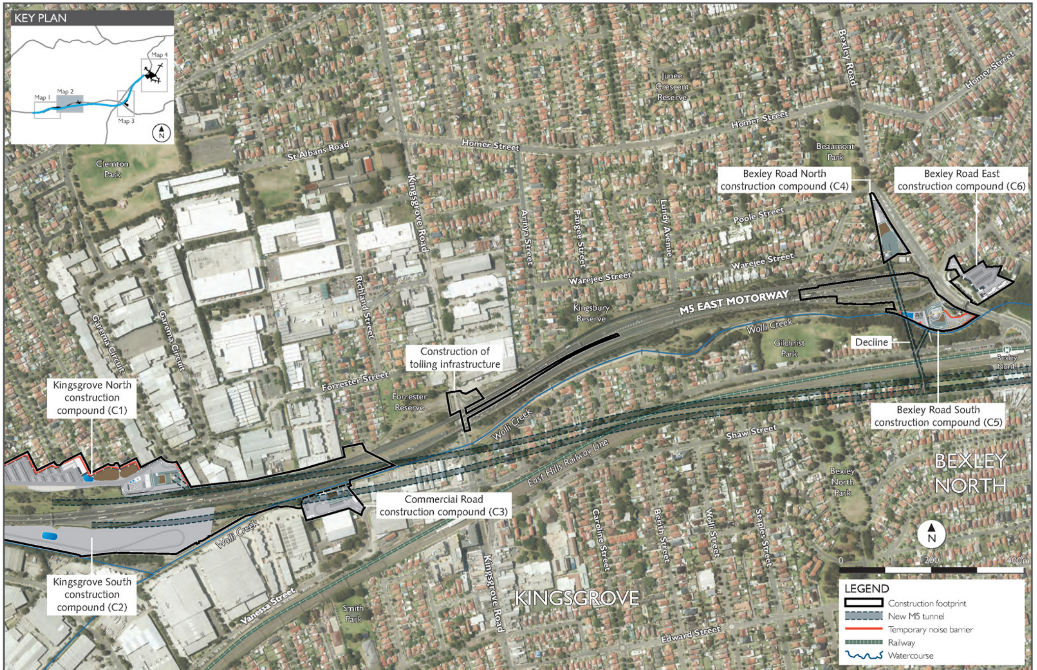
Figure 6-2 Project construction footprint - map 2
