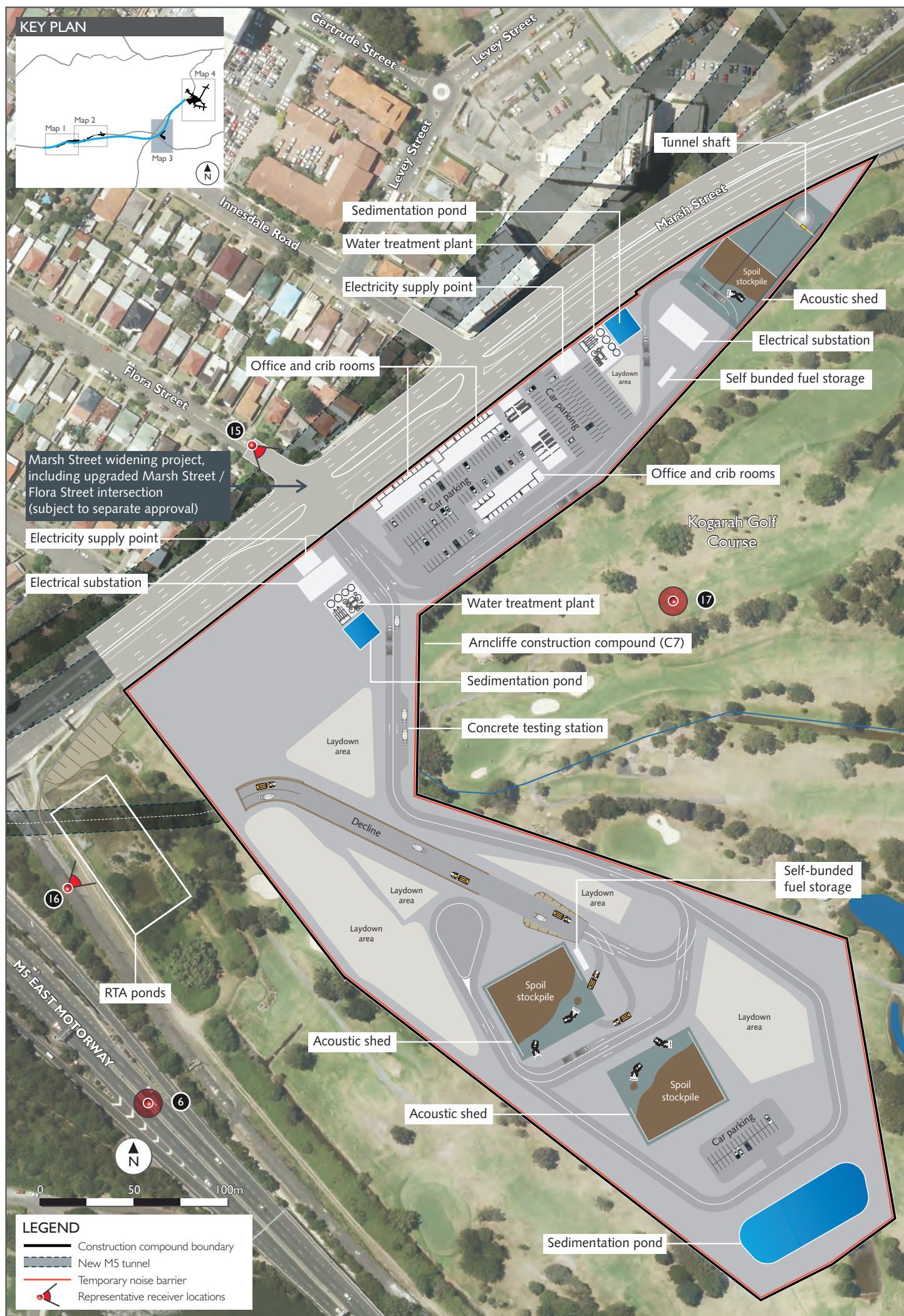
Figure 6-24 Arncliffe construction compound and receiver locations
