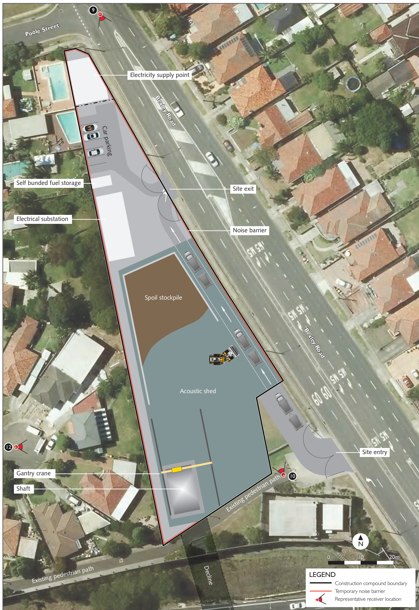
Figure 6-12 Bexley Road North construction compound and receiver locations
