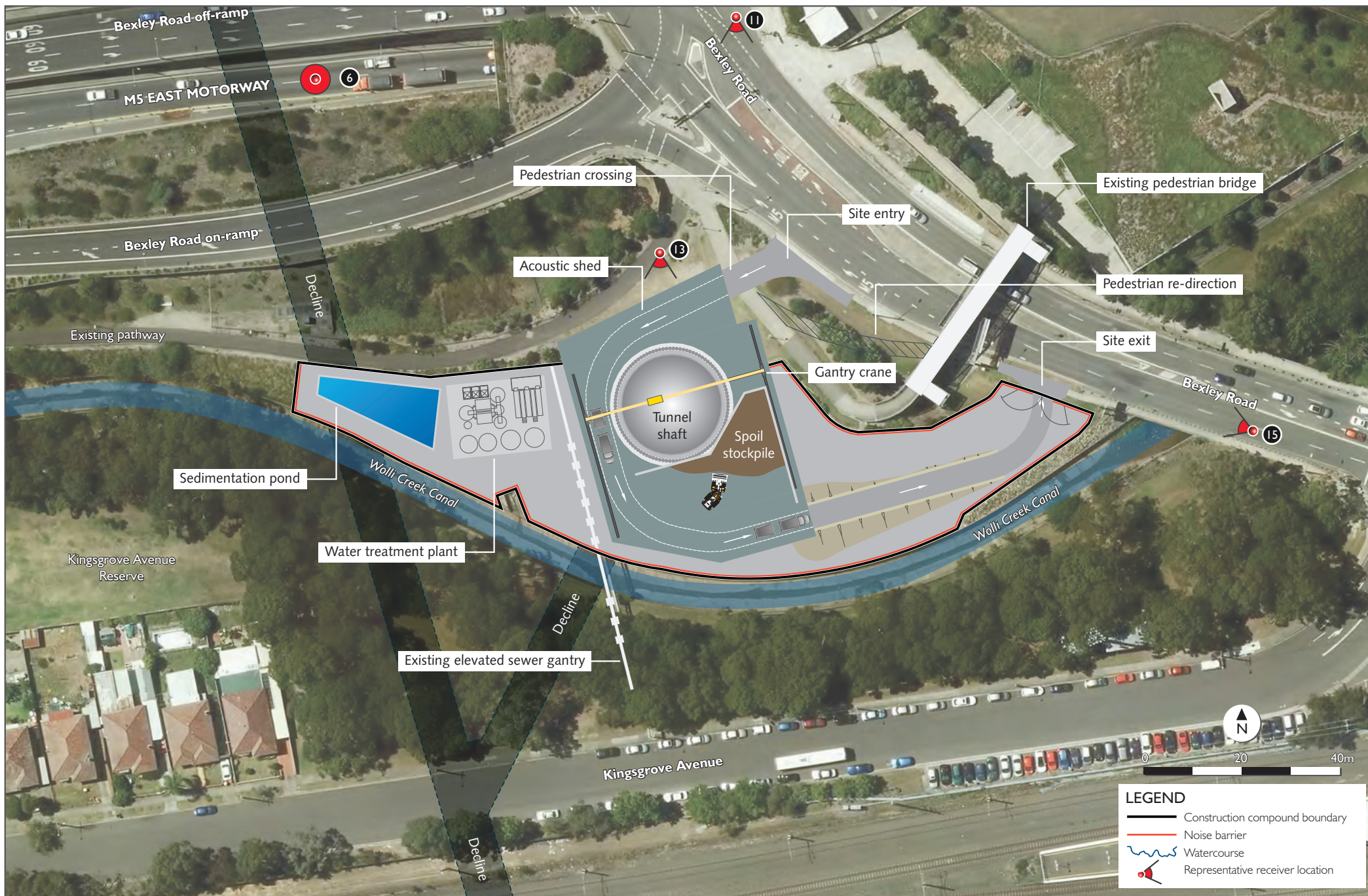
Figure 6-19 Bexley Road South construction compound and receiver locations
