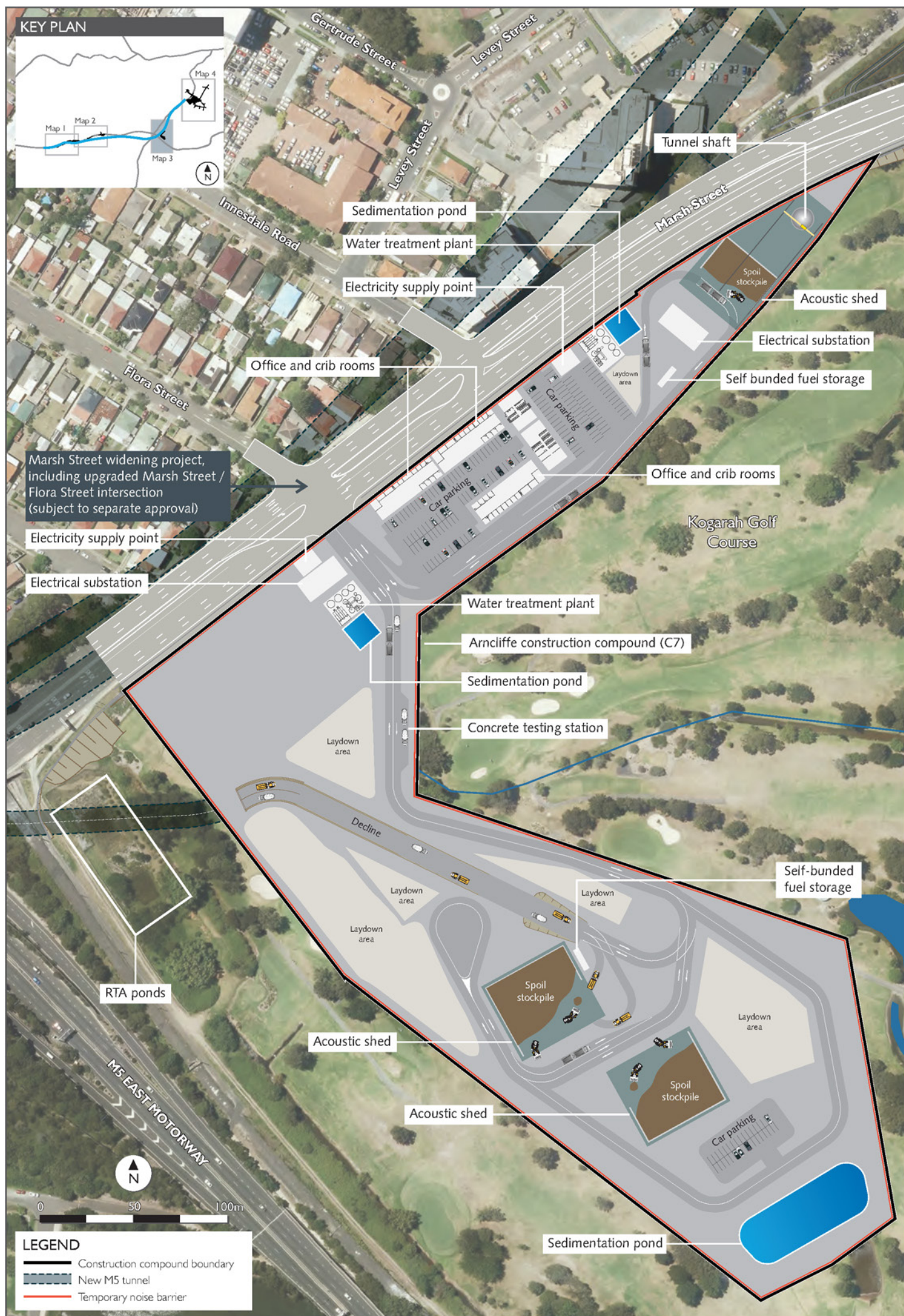
Figure 6-12 Indicative Arncliffe construction compound (C7) layout
