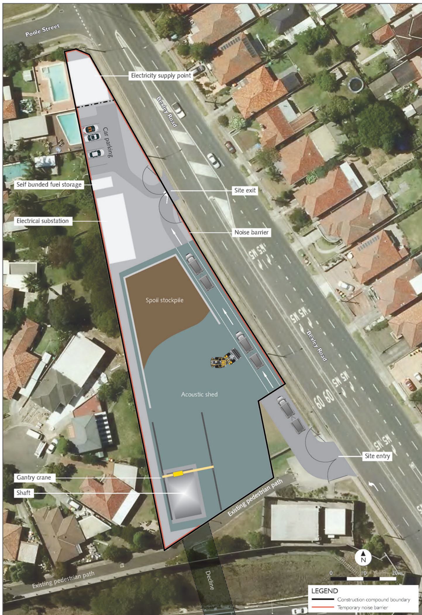
Figure 6-9 Bexley Road North construction compound (C4) layout
