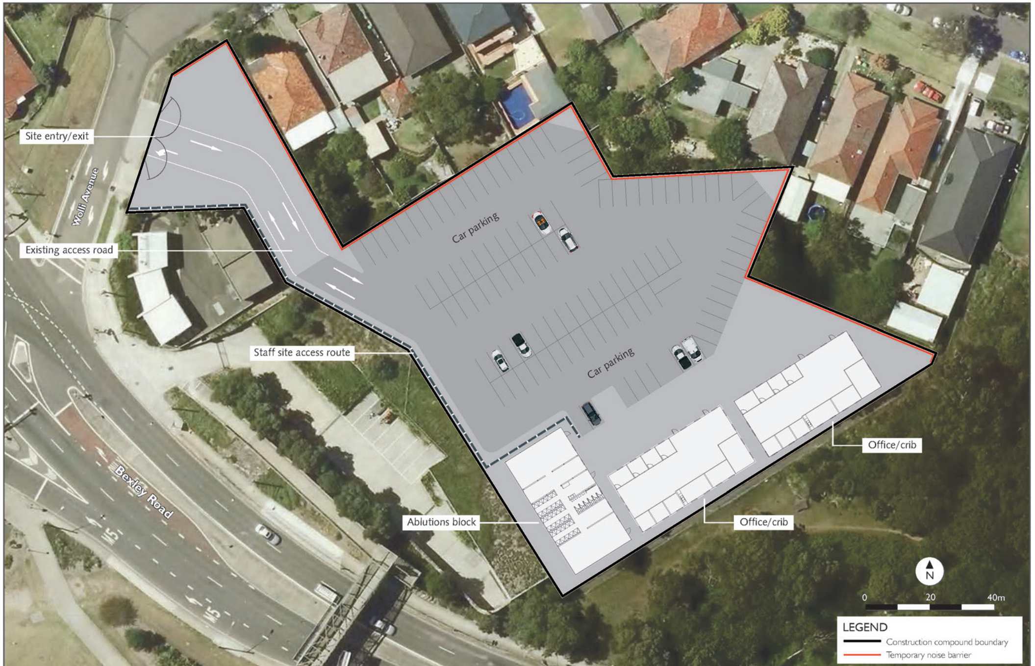
Figure 6-11 Bexley Road East construction compound (C6) layout
