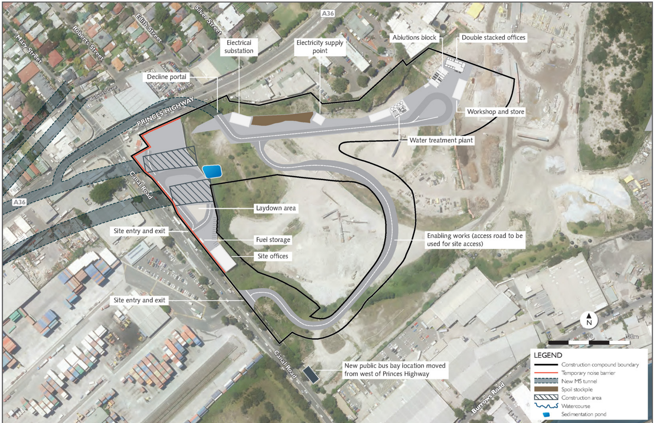
Figure 6-13 Canal Road construction compound (C8) layout
