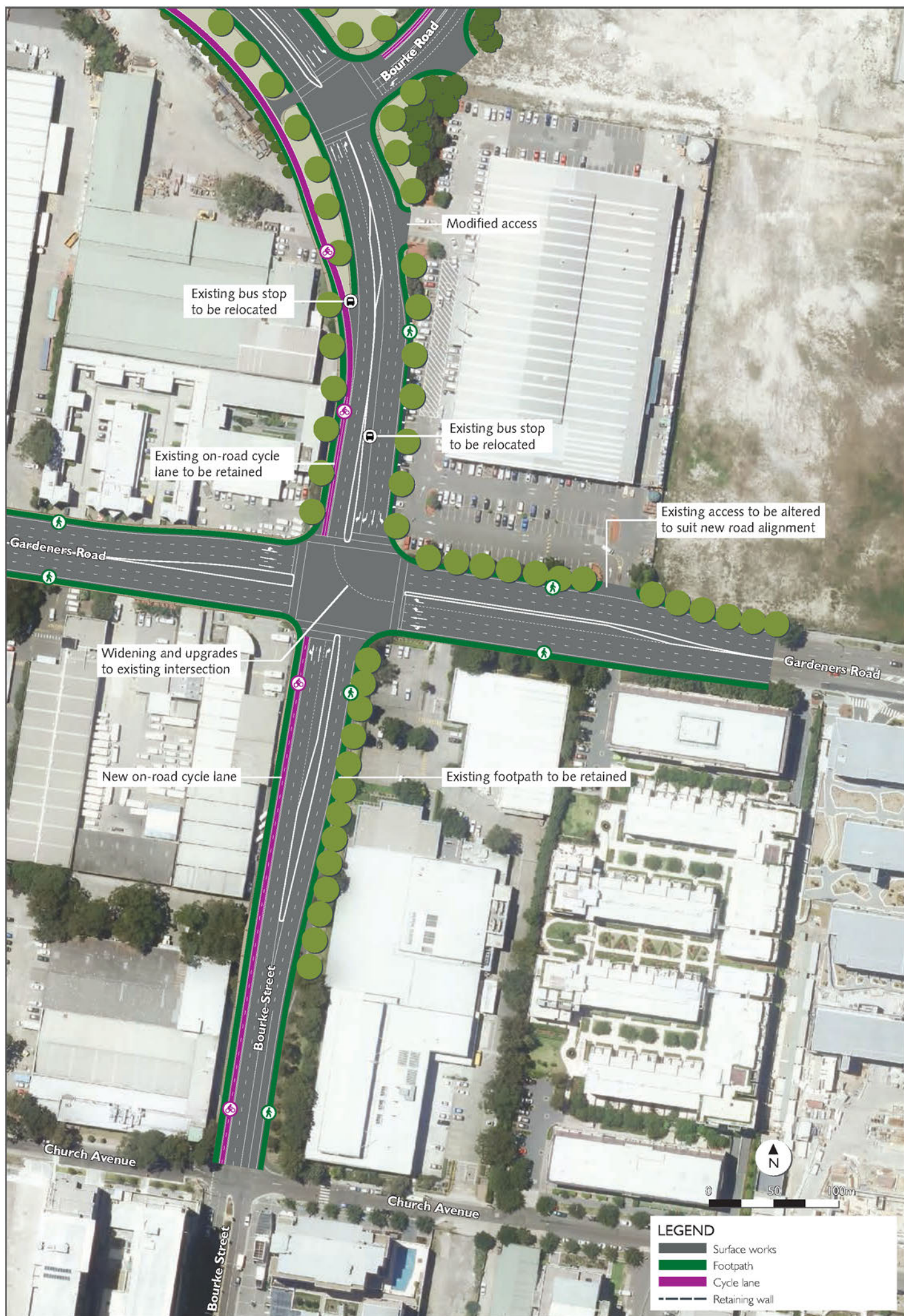
Figure 5-35 Bourke Road / Bourke Street widening and upgrade works
