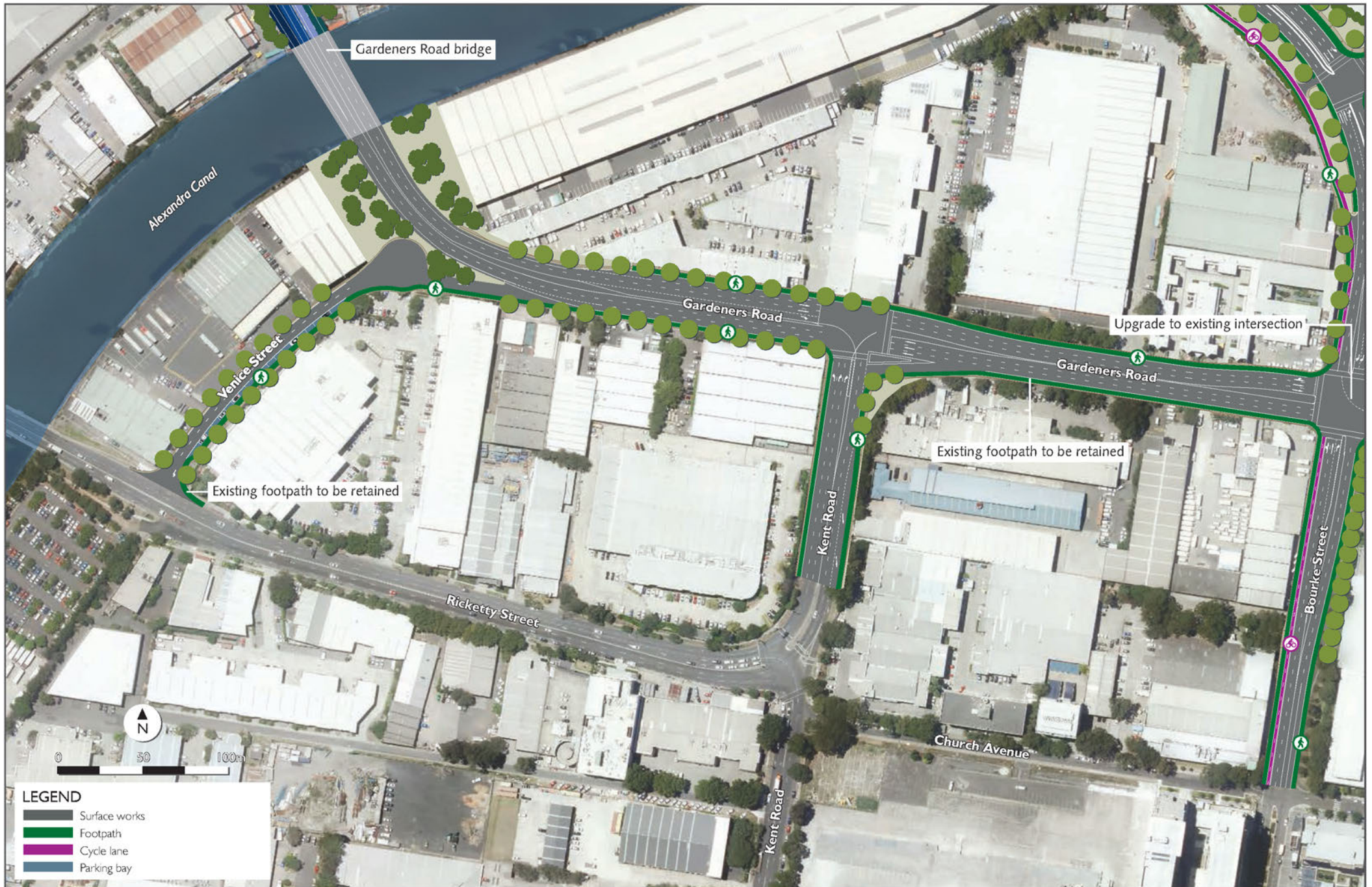
Figure 5-36 Gardeners Road upgrade and widening works
