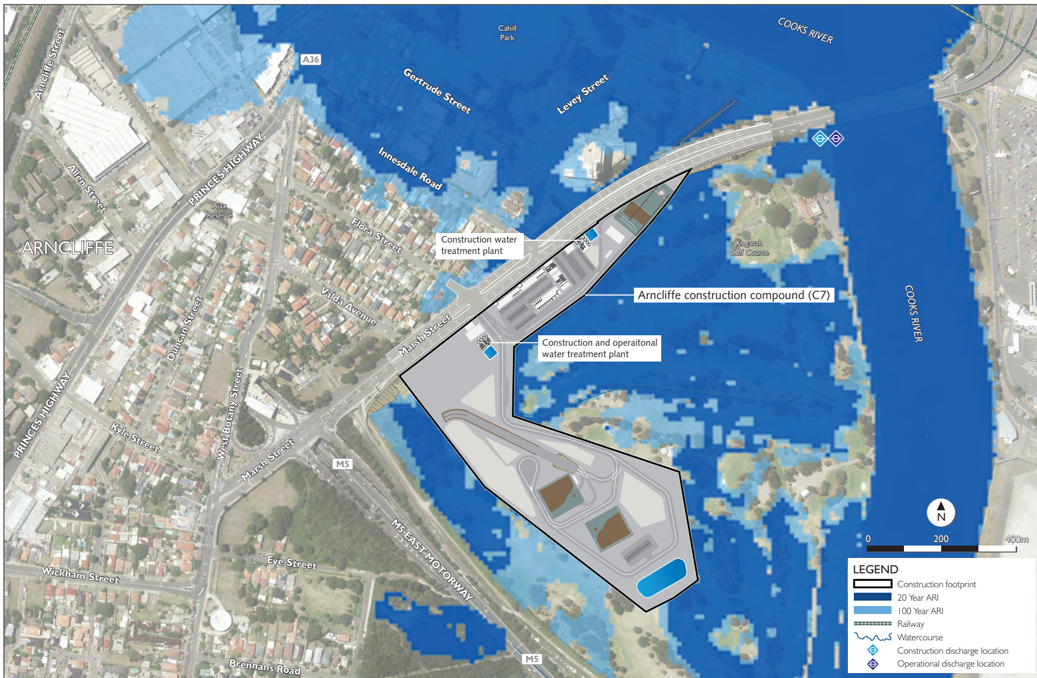
Figure 15 Modelled flood extents - Arncliffe construction compound
