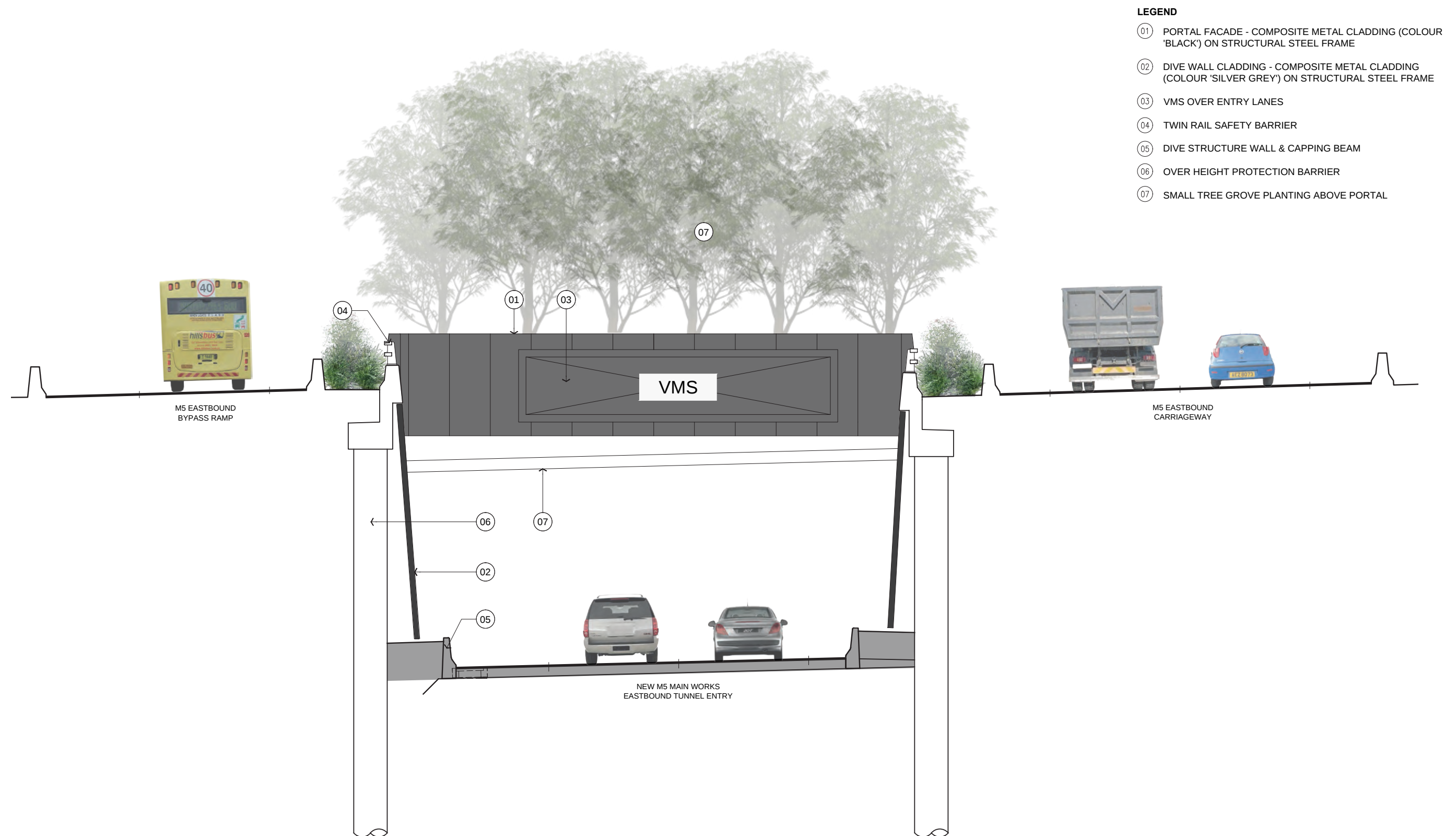
01 SECTION ELEVATION - TUNNEL PORTAL ENTRY 1:100
