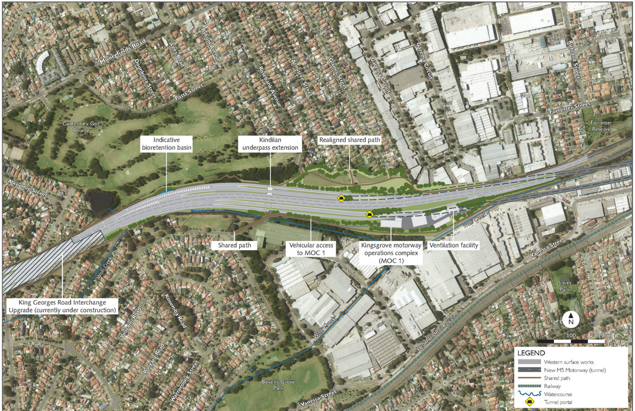
Figure 5-9 Overview of Western surface works
