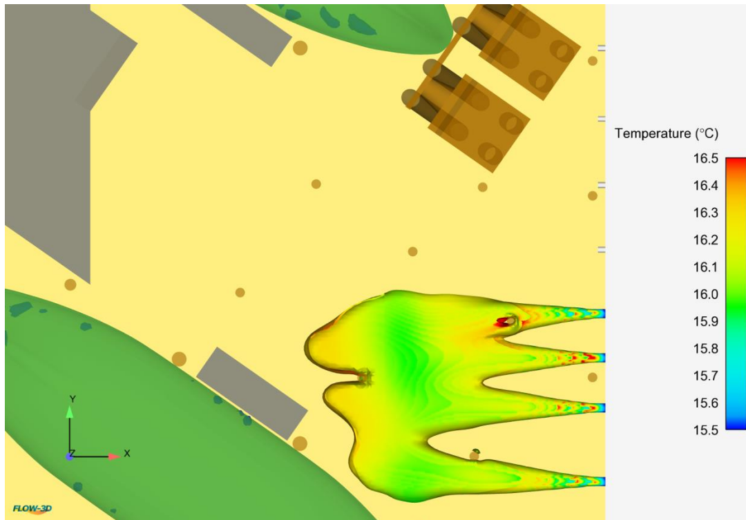
Figure 39: Winter – near field isosurface (velocity magnitude of 0.2 m/s) coloured by temperature, plan view
