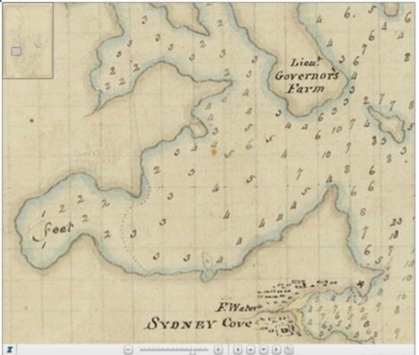
Figure 2: Extract from John Hunter's Chart of Port Jackson as surveyed in 1788. Image shows the shoreline and depth of water in Darling Harbour including the study area. Image courtesy: State Library of NSW (Z/M2 811.15/1788/1).
