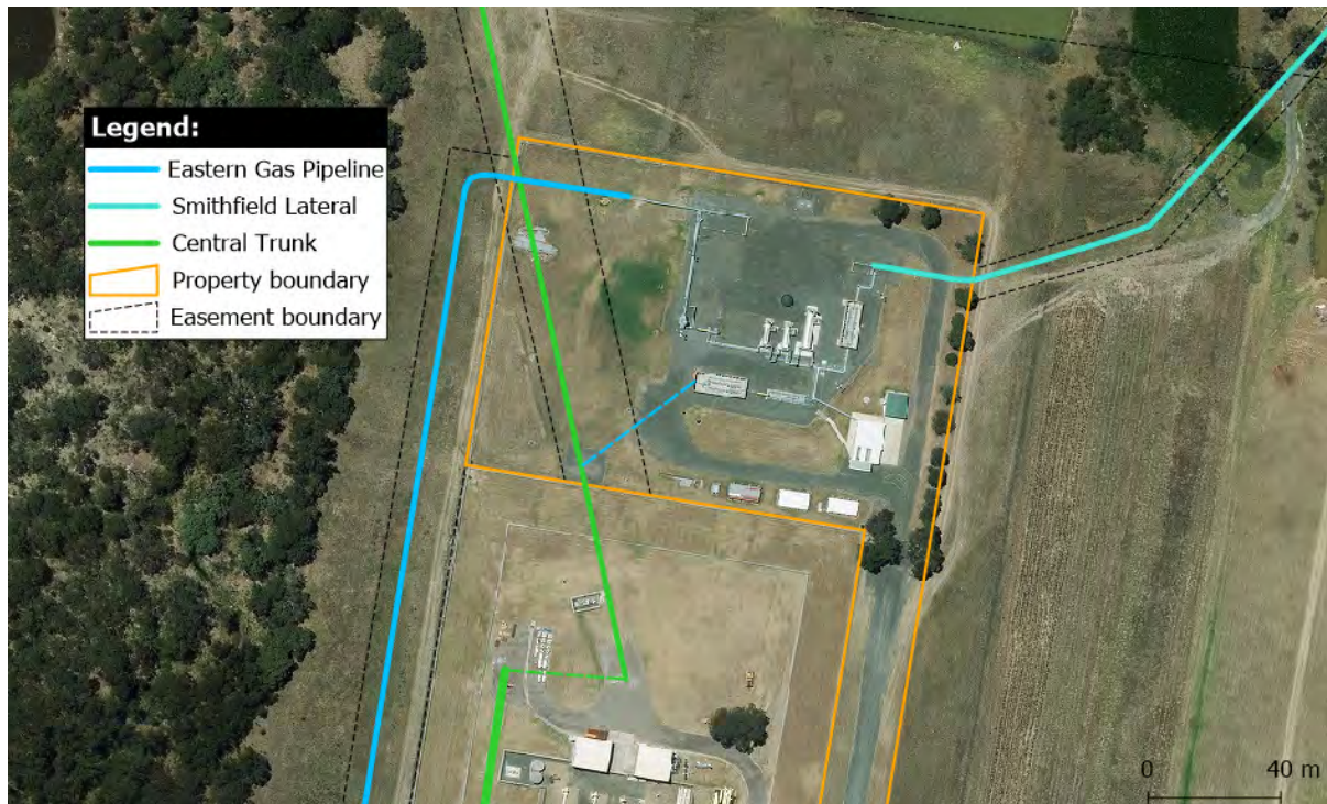
Figure 1-4 Pipelines connected by the Horsley Park Meter Station
