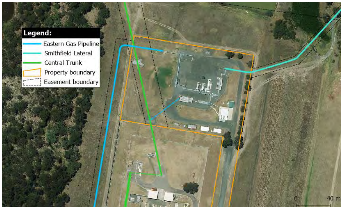
Figure 3 – Pipelines connected by the HPMS
